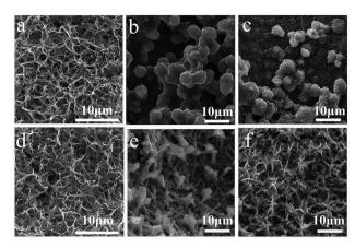
Fig. 6 SEM images of  $Co_3O_4$  (a) at the initial state, (b) after the  $10^{th}$  discharge and (c) after the  $10^{th}$  charge. SEM images of  $RuO_2-Co_3O_4$  (d) at the initial state, (e) after the  $10^{th}$  discharge and (f) after the  $10^{th}$  charge.
