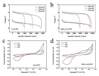
Fig. 3 (a and b) First discharge/charge curves of the  $Co_3O_4$ -catalyzed and  $RuO_2-Co_3O_4$ -catalyzed  $Li-O_2$  batteries at different current densities with a terminal voltage of 2.0-4.2 V. (c and d) CV curves of the  $Co_3O_4$ -catalyzed and  $RuO_2-Co_3O_4$ -catalyzed  $Li-O_2$  batteries at 2.0-4.3 V.
