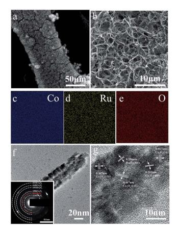
Fig. 2 (a and b) SEM images and (c–e) EDXS mapping of  $RuO_2-Co_3O_4$  nanowires on Ni foam, (f) TEM image with an inset showing the selected area electron diffraction (SAED) pattern and (g) the HRTEM image of  $RuO_2-Co_3O_4$  exfoliated from the Ni foam.
