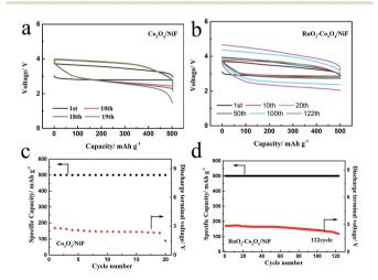
Fig. 4 Voltage profiles and cycling performances of (a and c)  $Co_3O_4$ -catalyzed as well as (b and d)  $RuO_2-Co_3O_4$ -catalyzed  $Li-O_2$  batteries at a current density of 100 mA  $g^{-1}$  with limited capacities of 500 mA h  $g^{-1}$ .
