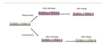
Fig. 5 Schematic illustrations of the formation of discharge products on the surfaces of  $Co_3O_4$  nanowires and  $RuO_2-Co_3O_4$  nanowires.
