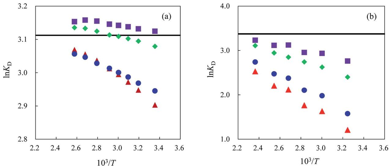
Fig. 5 Plots of  $\ln K_D$  for alkali metal ions as a function of reciprocal of temperature on a MCI GEL CK02A column (a) and a Nafion column (b). Eluent: 25 mM  $\text{Cs}_2\text{SO}_4$ . Symbols: ( $\blacktriangle$ )  $\text{Li}^+$ , ( $\bullet$ )  $\text{Na}^+$ , ( $\blacklozenge$ )  $\text{K}^+$ , ( $\blacksquare$ )  $\text{Rb}^+$ . The solid line denotes the  $\ln K_D(E)$  value for each column.
