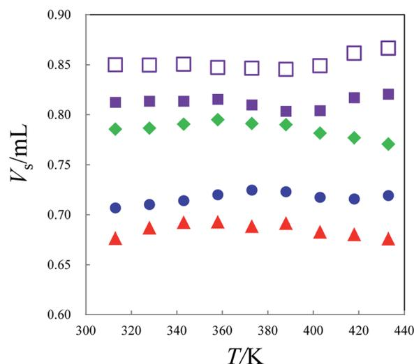
Fig. 8 Dependence of the  $V_s$  values on temperature for MCI GEL CK10S resin in alkali metal ion forms. For other details see Fig. 7.
