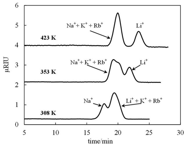
Fig. 3 Chromatograms of alkali metal ions on a MCI GEL CK10S column (4.6 mm I.D.  $\times$  50 mm) obtained at 308 K, 353 K and 423 K. Eluent: 25 mM  $\text{Cs}_2\text{SO}_4$ . Detection: differential refractometer. Flow rate: 1.5 mL  $\text{min}^{-1}$ .
