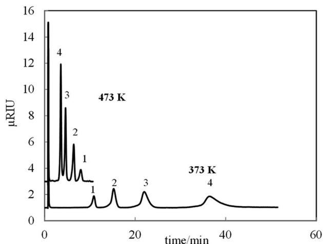
Fig. 4 Chromatograms of tetraalkylammonium ions on a MCI GEL CK10S column (4.6 mm I.D.  $\times$  50 mm) obtained at 373 K and 473 K. Eluent: 25 mM  $\text{Cs}_2\text{SO}_4$ . Detection: differential refractometer. Flow rate: 1.8 mL  $\text{min}^{-1}$ . Analyte: 1 = tetramethylammonium ion, 2 = tetraethylammonium ion, 3 = tetra-*n*-propylammonium ion, 4 = tetra-*n*-butylammonium ion.
