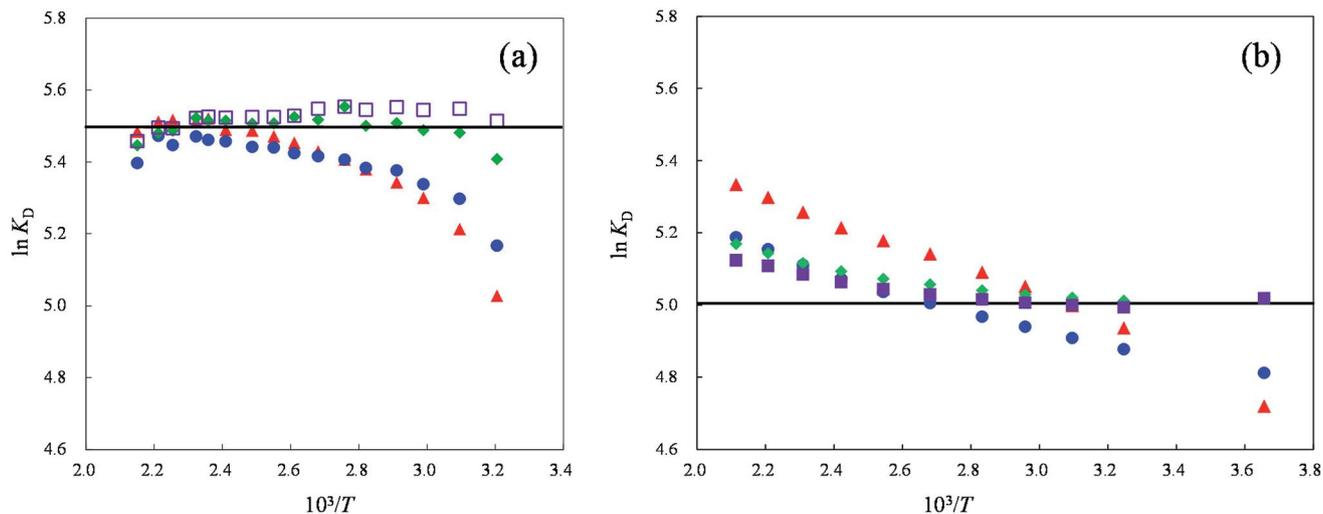
Fig. 1 Plots of  $\ln K_D$  for alkali metal ions as a function of reciprocal of temperature on a MCI GEL CK10S column. Eluent: (a) 25 mM  $\text{Rb}_2\text{SO}_4$ , (b) 25 mM  $\text{Cs}_2\text{SO}_4$ . Symbols: ( $\blacktriangle$ )  $\text{Li}^+$ , ( $\bullet$ )  $\text{Na}^+$ , ( $\blacklozenge$ )  $\text{K}^+$ , ( $\blacksquare$ )  $\text{Rb}^+$ , ( $\square$ )  $\text{Cs}^+$ . The solid line denotes the  $\ln K_D(E)$  value for each column.
