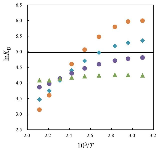
Fig. 2 Plots of  $\ln K_D$  for tetraalkylammonium ions as a function of reciprocal of temperature on a MCI GEL CK10S column. Eluent: 25 mM  $\text{Cs}_2\text{SO}_4$ . ( $\blacktriangle$ ) tetramethylammonium ion, ( $\bullet$ ) tetraethylammonium ion, ( $\blacklozenge$ ) tetra-*n*-propylammonium ion, ( $\bullet$ ) tetra-*n*-butylammonium ion. The solid line denotes the  $\ln K_D(E)$  value.
