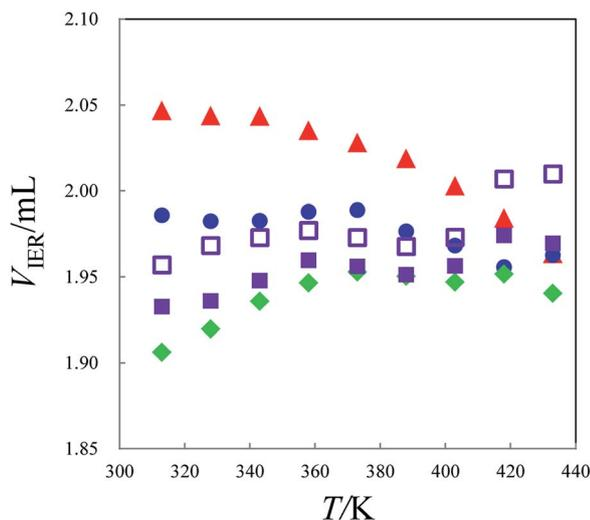
Fig. 7 Dependence of the  $V_{IER}$  values on temperature for MCI GEL CK10S resin in alkali metal ion forms. Symbols: (▲)  $\text{Li}^+$ , (●)  $\text{Na}^+$ , (◆)  $\text{K}^+$ , (■)  $\text{Rb}^+$ , (□)  $\text{Cs}^+$ .
