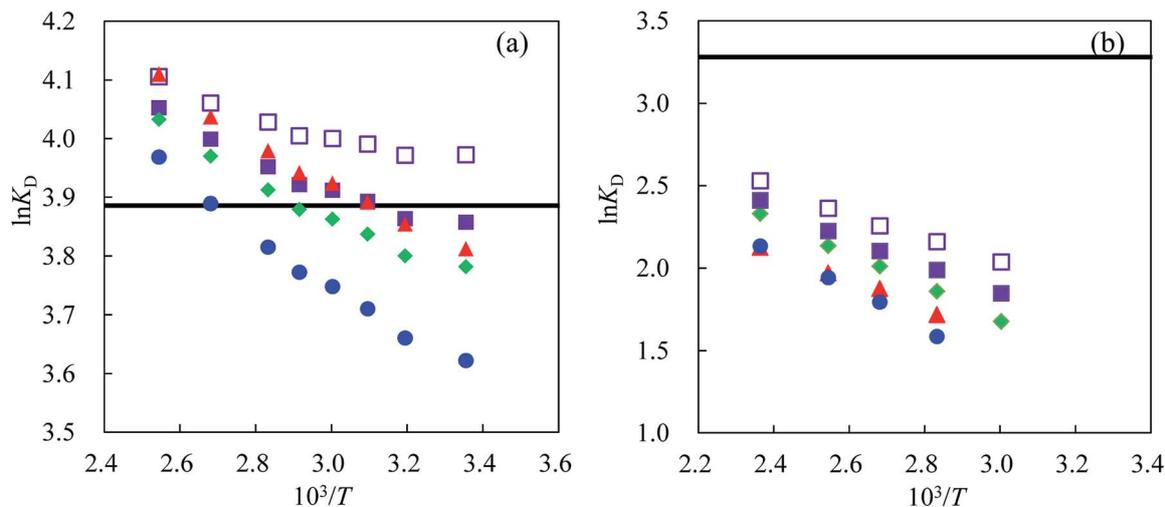
Fig. 6 Plots of  $\ln K_D$  for alkali metal ions as a function of reciprocal of temperature on a MCI GEL CK02A column (a) and a Nafion column (b). Eluent: 50 mM TMABr. Symbols: (▲)  $\text{Li}^+$ , (●)  $\text{Na}^+$ , (◆)  $\text{K}^+$ , (■)  $\text{Rb}^+$ , (□)  $\text{Cs}^+$ . The solid line denotes the  $\ln K_D(E)$  value for each column.
