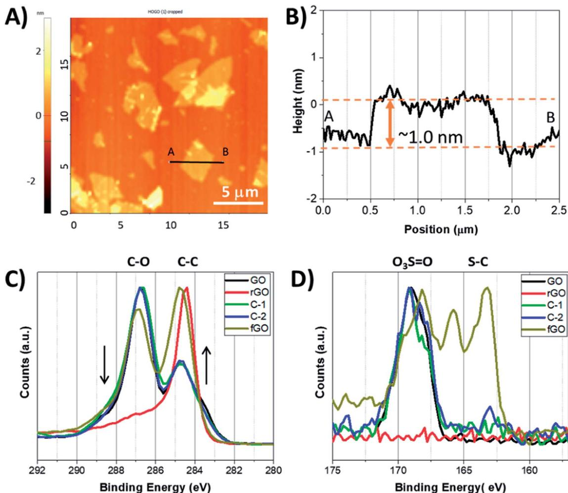
Fig. 1 A) AFM image of GO nanosheets prepared by drop-casting an aqueous dispersion onto mica substrate; (B) Line profile of GO nanosheet indicated in A; (C) C 1s high resolution XPS scan; (D) S 2p<sub>3/2</sub> high resolution XPS scan. GO (black trace), rGO (red trace), fGO (olive trace), C-1 (green), and C-2 (blue).
