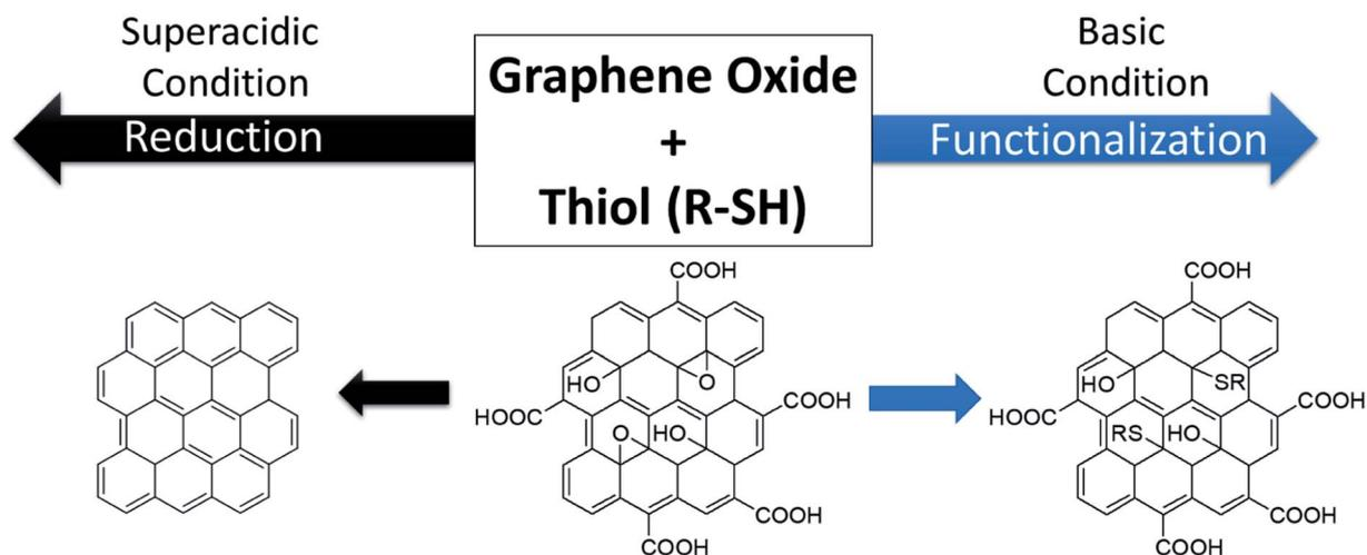
**Scheme 1** Overview of the work reported herein: in the presence of ethane thiol (EtSH), graphene oxide (GO) nanosheets can be reduced in a superacidic solution, or functionalized in a basic solution.
