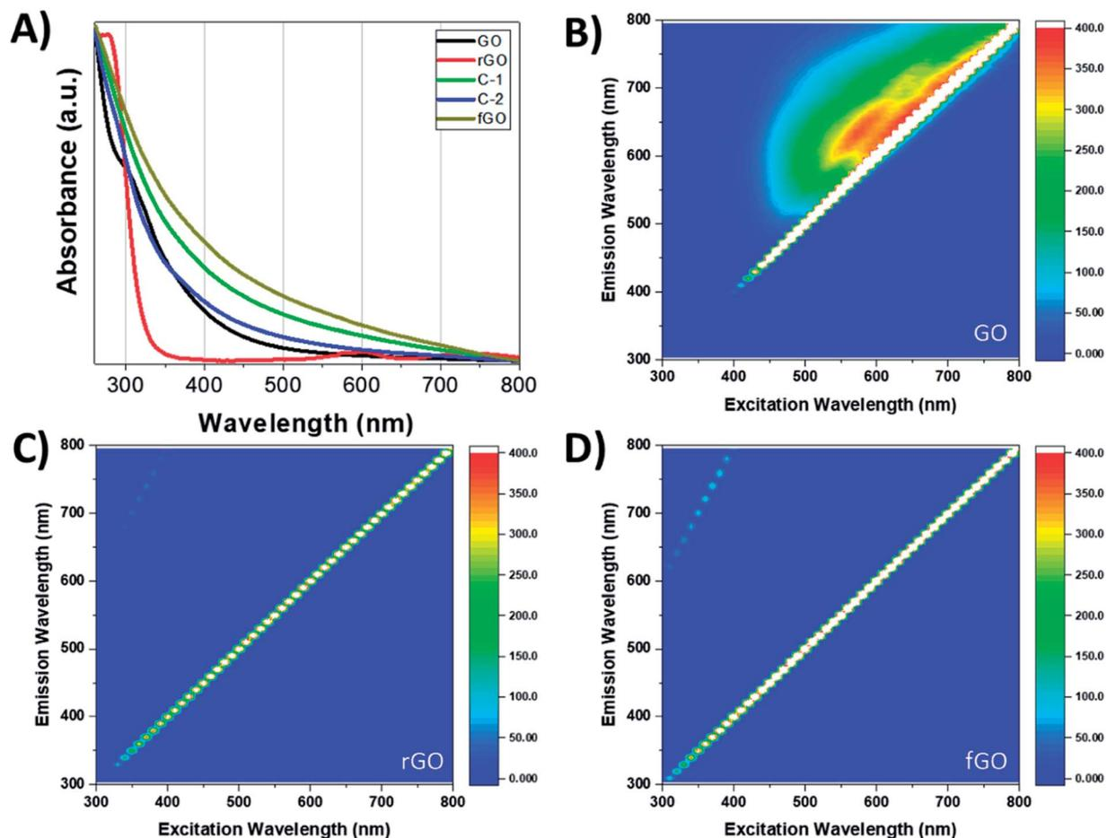
Fig. 4 (A) UV-Vis spectra of GO, rGO, fGO, C-1, and C-2 suspended in DMSO; 2D fluorescence spectra of (B) GO; (C) rGO; and (D) fGO.
