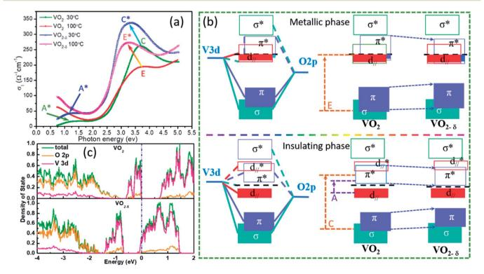
Fig. 4 The optical conductivity curves of  $VO_2$  and  $VO_{2-\delta}$  at room temperature and 100 °C (a), the schematic band structure of  $VO_2$  or  $VO_{2-\delta}$  in metallic and insulating state (b), the density of state  $VO_2$  and  $VO_{2-\delta}$  based on first principle calculation (c).
