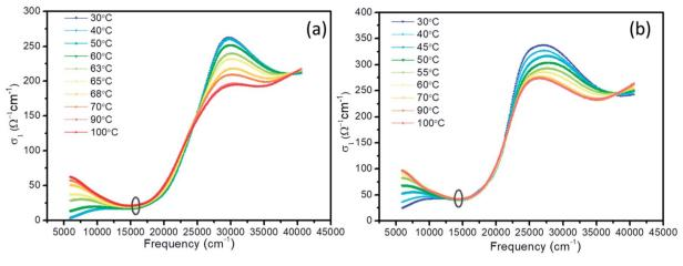
Fig. 3 Optical conductivity of VO<sub>2</sub> (a) and VO<sub>2- $\delta$ </sub> (b) films as a function of wavenumber at representative temperature.
