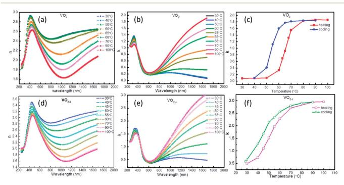
Fig. 2 The n (a and d) and k (b and e) of VO<sub>2</sub> and VO<sub>2- $\delta$ </sub> films as a function of wavelength under different temperature, the k-T curves (c and f) of  $VO_2$  and  $VO_{2-\delta}$ .
