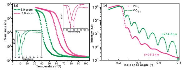
Fig. 1 Thermal hysteresis loops of VO<sub>2</sub> and VO<sub>2- $\delta$ </sub> films (a), inset shows the differential curve of R-T, XRR curves of VO<sub>2</sub> and VO<sub>2- $\delta$ </sub> with the 10 keV X-ray incidence (b).
