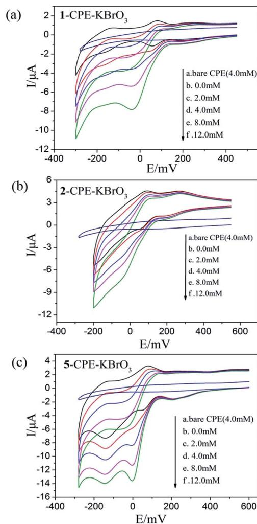
Fig. 7 Cyclic voltammograms of the 1-CPE, 2-CPE and 5-CPE in 0.1 M H<sub>2</sub>SO<sub>4</sub> + 0.5 M Na<sub>2</sub>SO<sub>4</sub> aqueous solution containing 0.0–12.0 mM KBrO<sub>3</sub>.
