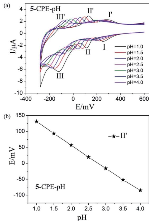
Fig. 9 (a) Cyclic voltammograms of 5-CPE at different pH values (Scan rate:  $40 \text{ mV s}^{-1}$ ); (b) Variation of anodic peak potentials of the  $\text{Mo}^{\text{VI}}$ -based wave (II') with different pH for 5-CPE.
