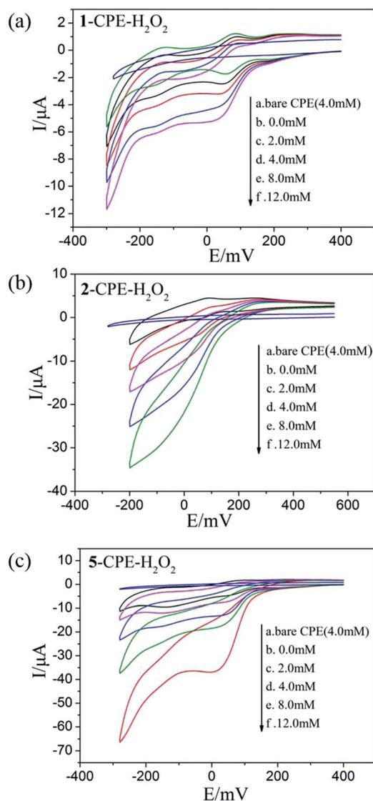
Fig. 6 Cyclic voltammograms of the 1-CPE, 2-CPE and 5-CPE in 0.1 M H<sub>2</sub>SO<sub>4</sub> + 0.5 M Na<sub>2</sub>SO<sub>4</sub> aqueous solution containing 0.0–12.0 mM H<sub>2</sub>O<sub>2</sub>.
