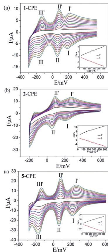
Fig. 5 Cyclic voltammograms of the (a) 1-CPE (b) 2-CPE (c) 5-CPE in 0.1 M H<sub>2</sub>SO<sub>4</sub> + 0.5 M Na<sub>2</sub>SO<sub>4</sub> aqueous solution under scan rates from inner to outer: (scan rates: 40, 80, 120, 160, 200, 250, 300, 350, 400, 450, 500 mV s<sup>-1</sup>). Inset: the dependence of cathodic peak and anodic peak currents on scan rates of 1-, 2- and 5-CPEs.
