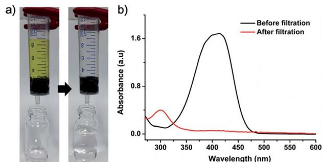
Fig. 8 (a) Sequential photographs showing the 4-NP reduction reaction with Pd-CMP<sub>300</sub> and (b) UV-Vis spectra of the 4-NP stock solution and the filtered solution.
