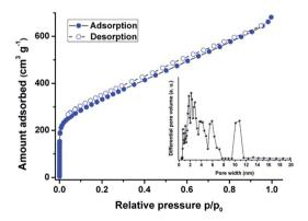
Fig. 6 N<sub>2</sub> adsorption-desorption isotherms measured at 77 K and NL-DFT pore size distribution of the Pd-CMP (inset).
