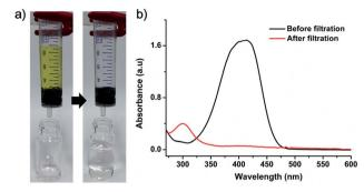
Fig. 8 (a) Sequential photographs showing the 4-NP reduction reaction with Pd-CMP $_{300}$  and (b) UV-Vis spectra of the 4-NP stock solution and the filtered solution.
