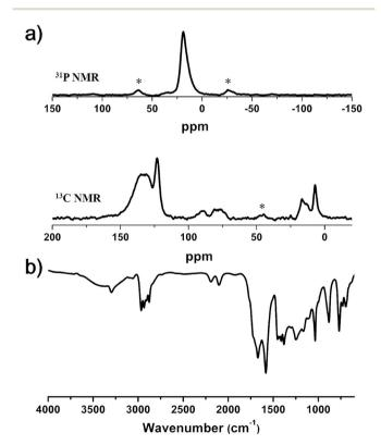
Fig. 5 (a) Solid-state <sup>31</sup>P (up) and <sup>13</sup>C (down) CP/MAS NMR spectra and (b) FT-IR spectrum of Pd-CMP (asterisks denote spinning sidebands).
