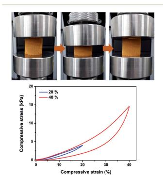
Fig. 2 Photo images of the Pd-CMP monolith taken during the compression test and the compressive stress-strain curves (maximum strain = 20 and 40%
