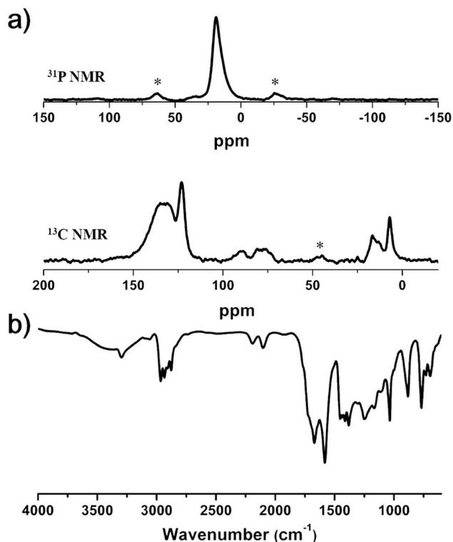
Fig. 5 (a) Solid-state <sup>31</sup>P (up) and <sup>13</sup>C (down) CP/MAS NMR spectra and (b) FT-IR spectrum of Pd-CMP (asterisks denote spinning sidebands).
