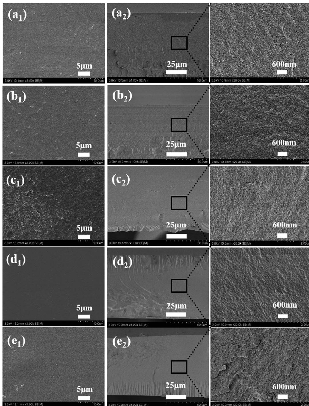
Fig. 2 Surface ( $a_1$ ,  $b_1$ ,  $c_1$ ,  $d_1$  and  $e_1$ ) and cross-section morphology ( $a_2$ ,  $b_2$ ,  $c_2$ ,  $d_2$  and  $e_2$ ) of BSF/TSF blend films with various blend ratios. ( $a_1$  and  $a_2$ ) BSF, ( $b_1$  and  $b_2$ ) 3/1, ( $c_1$  and  $c_2$ ) 1/1, ( $d_1$  and  $d_2$ ) 1/3, ( $e_1$  and  $e_2$ ) TSF.
