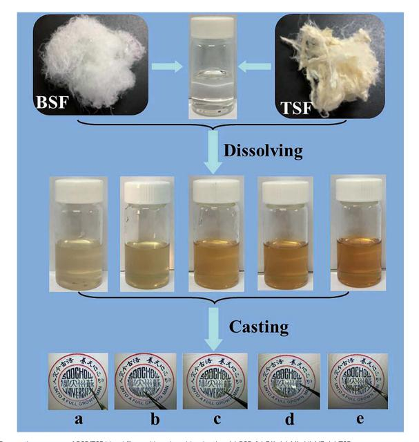
Fig. 1 Preparation process of BSF/TSF blend films with various blend ratios. (a) BSF, (b) 3/1, (c) 1/1, (d) 1/3, (e) TSF.
