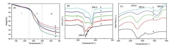
Fig. 5 TGA (A), DTG (B) and DSC (C) curves of BSF/TSF blend films with various blend ratios. (a) BSF, (b) 3/1, (c) 1/1, (d) 1/3, (e) TSF, nitrogen flux at  $30 \text{ ml min}^{-1}$ , heating rate at  $10 ^{\circ}\text{C}$  min $^{-1}$  and temperature range from  $50 \text{ to } 600 ^{\circ}\text{C}$ , and the samples weight was about 5 mg.
