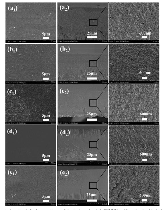
Fig. 2 Surface  $(a_1, b_1, c_1, d_1 \text{ and } e_1)$  and cross-section morphology  $(a_2, b_2, c_2, d_2 \text{ and } e_2)$  of BSF/TSF blend films with various blend ratios.  $(a_1 \text{ and } a_2)$  BSF,  $(b_1 \text{ and } b_2)$  3/1,  $(c_1 \text{ and } c_2)$  1/1,  $(d_1 \text{ and } d_2)$  1/3,  $(e_1 \text{ and } e_2)$  TSF.
