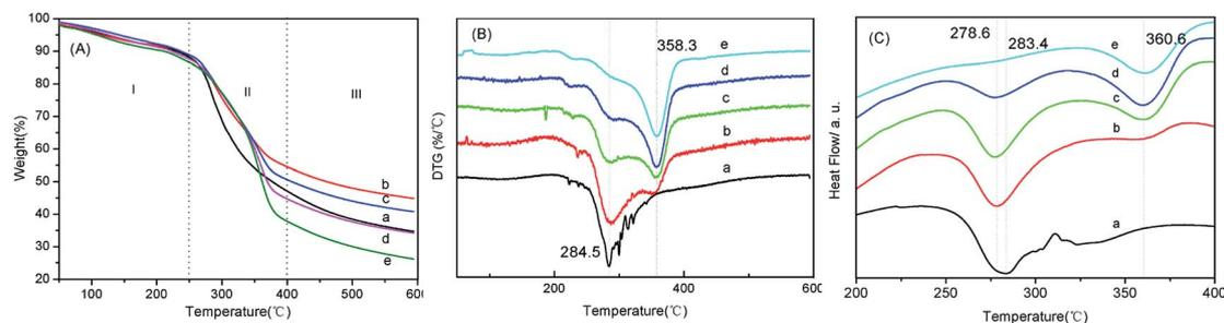
Fig. 5 TGA (A), DTG (B) and DSC (C) curves of BSF/TSF blend films with various blend ratios. (a) BSF, (b) 3/1, (c) 1/1, (d) 1/3, (e) TSF, nitrogen flux at  $30\text{ ml min}^{-1}$ , heating rate at  $10\text{ }^\circ\text{C min}^{-1}$  and temperature range from 50 to  $600\text{ }^\circ\text{C}$ , and the samples weight was about 5 mg.
