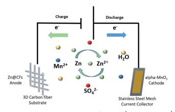
Fig. 1 Schematic illustration of Zn@CFs|2.0 mol  $l^{-1}$  ZnSO<sub>4</sub>, 0.1 mol  $l^{-1}$  MnSO<sub>4</sub>| $\alpha$ -MnO<sub>2</sub> aqueous battery.
