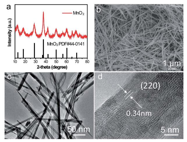
Fig. 5 Characterizations of  $\alpha$ -MnO<sub>2</sub> nanowire cathode. (a) XRD patterns of the as-prepared  $\alpha$ -MnO<sub>2</sub>, (b) SEM image, (c) TEM image and (d) magnified TEM image.
