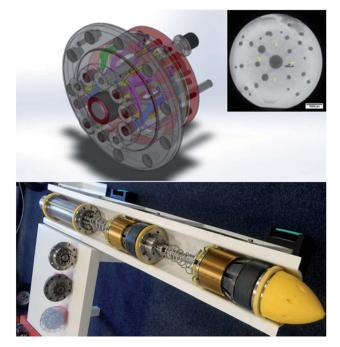
Fig. 11 The CAD design of the gateway manifold with complex internal channels (top), cross section showing the fine resolution and small feature sizes enabled by additive manufacturing (inset) and the product at each stage along the manufacturing process and deployed in the assembled pipeline isolation tool (bottom).
