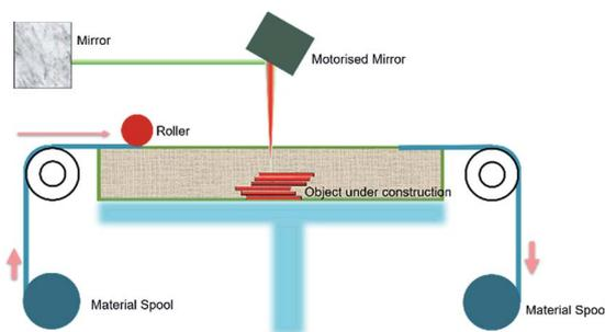
Fig. 5 Schematic diagram showing the sheet lamination process.
