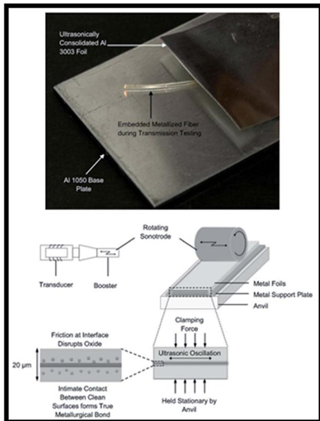
Fig. 10 The incorporation of a fiber optic cable in an additively manufactured structure (top) and processing schematic (bottom).
