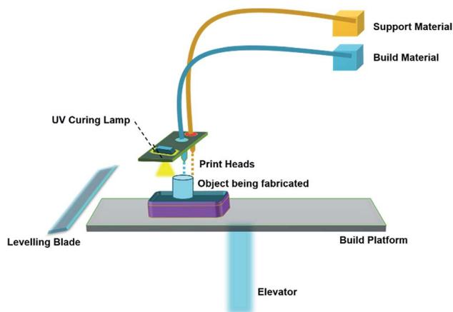
Fig. 3 Schematic representation of the material jetting process.
