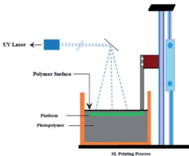
Fig. 1 Schematic representation of the SL printing process.
