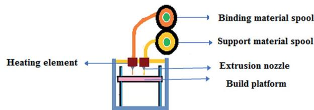
Fig. 2 Schematic representation of the fused deposition process.
