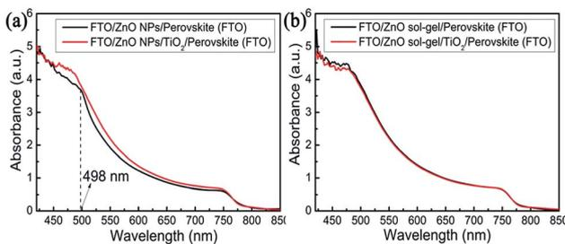
Fig. 8 Absorbance spectra of perovskite films deposited (a) on a ZnO NP-film and a ZnO NPs/TiO<sub>2</sub> bilayered film; (b) on a ZnO sol-gel film and a ZnO sol-gel/TiO<sub>2</sub> bilayered film.
