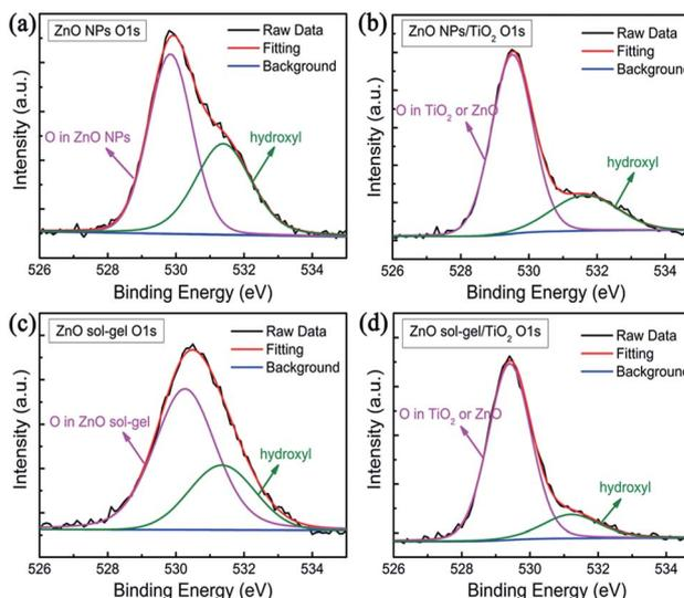
Fig. 3 XPS spectra of (a) a ZnO-NP film, (b) a ZnO NPs/TiO<sub>2</sub> bilayered film, (c) a ZnO sol-gel film, and (d) a ZnO sol-gel/TiO<sub>2</sub> bilayered film.
