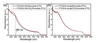
Fig. 8 Absorbance spectra of perovskite films deposited (a) on a ZnO NP-film and a ZnO NPs/TiO<sub>2</sub> bilayered film; (b) on a ZnO sol-gel film and a ZnO sol-gel/TiO2 bilayered film.
