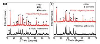
Fig. 7 XRD patterns of perovskite films deposited (a) on a ZnO-NP film and a ZnO NPs/TiO<sub>2</sub> bilayered film; (b) on a ZnO sol-gel film and a ZnO sol-gel/TiO2 bilayered film.
