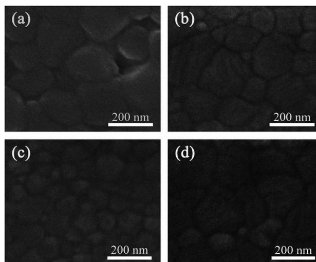
Fig. 5 SEM images of perovskite films deposited on (a) a ZnO-NP film, (b) a ZnO NPs/TiO<sub>2</sub> bilayered film, (c) a ZnO sol-gel film, and (d) a ZnO sol-gel/TiO<sub>2</sub> bilayered film, respectively.
