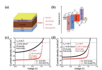
Fig. 6 (a) Schematic architecture of PSCs fabricated in the work; (b) schematic energy band diagram of PSCs fabricated in the work; typical J-V characteristics of perovskite solar cells fabricated (c) on a ZnO-NP film and a ZnO NPs/TiO<sub>2</sub> bilayered film; (d) on a ZnO sol-gel film and a ZnO sol-gel/TiO<sub>2</sub> bilayered film.
