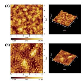
Fig. 4 Two and three dimensional AFM images of (a) a ZnO-NP film, (b) a ZnO sol-gel film.
