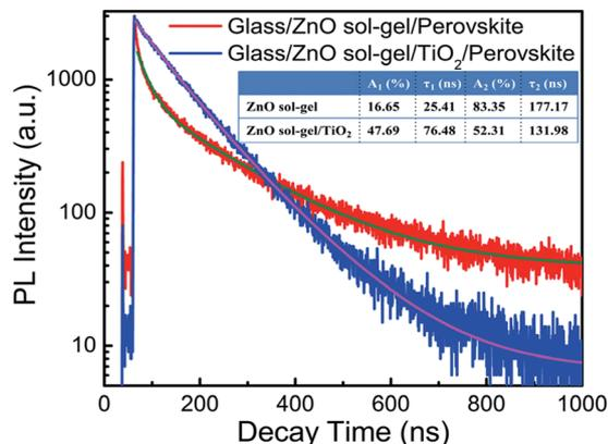
Fig. 9 Time resolved photoluminescence spectra of perovskite films deposited on a ZnO sol-gel film and a ZnO sol-gel/TiO<sub>2</sub> bilayered film. Inset: the resulting decay lifetimes ( $\tau_i$ ) and decay amplitudes ( $A_i$ ).
