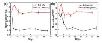
Fig. 10 Durability of perovskite solar cells fabricated (a) on a ZnO NP-film and a ZnO NPs/TiO $_2$  bilayered film; (b) on a ZnO sol–gel film and a ZnO sol–gel/TiO $_2$  bilayered film in air atmosphere (RH $\sim$ 20%).
