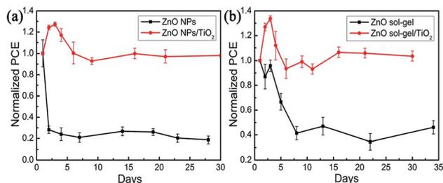
Fig. 10 Durability of perovskite solar cells fabricated (a) on a ZnO NP-film and a ZnO NPs/TiO<sub>2</sub> bilayered film; (b) on a ZnO sol-gel film and a ZnO sol-gel/TiO<sub>2</sub> bilayered film in air atmosphere (RH~20%).
