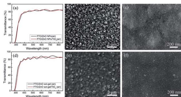
Fig. 1 Transmittance spectra (a and d) and SEM images of (b) a ZnO-NP film, (c) a ZnO NPs/TiO<sub>2</sub> bilayered film, (e) a ZnO sol-gel film, and (f) a ZnO sol-gel/TiO<sub>2</sub> bilayered film.
