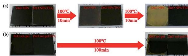
Fig. 2 The stability comparison between perovskite films deposited (a) on a ZnO-NP film and a ZnO NPs/TiO<sub>2</sub> bilayered film, (b) on a ZnO sol-gel film and a ZnO sol-gel/TiO<sub>2</sub> bilayered film upon thermal treatments.
