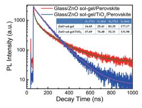
Fig. 9 Time resolved photoluminescence spectra of perovskite films deposited on a ZnO sol-gel film and a ZnO sol-gel/TiO<sub>2</sub> bilayered film. Inset: the resulting decay lifetimes  $(\tau_i)$  and decay amplitudes  $(A_i)$ .
