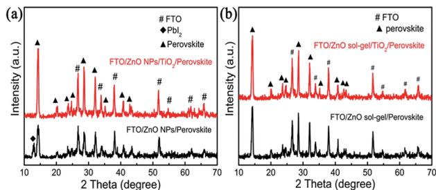
Fig. 7 XRD patterns of perovskite films deposited (a) on a ZnO-NP film and a ZnO NPs/TiO<sub>2</sub> bilayered film; (b) on a ZnO sol-gel film and a ZnO sol-gel/TiO<sub>2</sub> bilayered film.
