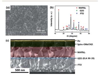
Fig. 5 (a) SEM image of MAPbl<sub>3</sub> layer on ELA 90-20. (b) XRD pattern of the MAPbl<sub>3</sub> film prepared on the ELA 90-20 at FTO substrate. (c) Cross-sectional SEM image of the cell employing ELA 90-20.
