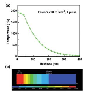
Fig. 4 (a) Temperature distribution along the film thickness when loading fluence of 90 mJ cm<sup>-2</sup> for 1 pulse (20 ns). (b) Temperature distribution in two dimensions model of ELA 90-20 at 20 ns.
