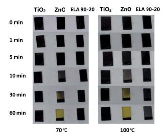
Fig. 8 Photographs of MAPbl<sub>3</sub> films deposited on different samples (TiO<sub>2</sub>, HZ and ELA 90-20 films) and heated to either 70 °C or 100 °C for the indicated time
