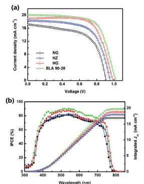
Fig. 6 (a) J-V curves and (b) IPCE spectra and integrated photocurrent density of the PHJ-PSC based on ZnO (blue, triangle), NG (black, diamond), HG (red, square), and ELA 90-20 (green, circle).
