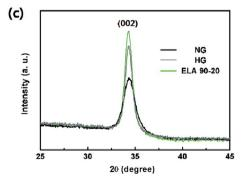
Fig. 2 (a) Variation of resistivity of ELA-treated GZO films with pulse counts (1, 5, 10, 20, and 40) under fluence at 60, 75, 90, and 105 mJ cm $^{-2}$ . (b) Transmittance spectra and (c) XRD patterns of NG, HG, and ELA 90-20 on glass.
