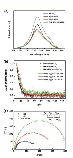
Fig. 7 (a) PL spectra of glass substrate/ETL/MAPbI<sub>3</sub> (ETL = NG, HG, ETL 90-20, or none) samples. (b) Transient absorption decay of glass substrate/ETL/MAPbl<sub>3</sub> (ETL = NG, HG, and ETL 90-20) samples. (c) Nyquist plots of the PHJ-PSCs based on NG, HG, and ELA 90-20. The inset is the equivalent circuit of the cell.
