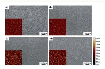
Fig. 3 SEM images of (a) glass substrate, (b) NG, (c) HG, and (d) ELA 90-20, the inset is the corresponding AFM image.
