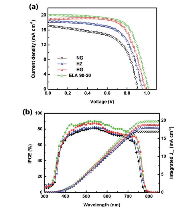
Fig. 6 (a) *J*-*V* curves and (b) IPCE spectra and integrated photocurrent density of the PHJ-PSC based on ZnO (blue, triangle), NG (black, diamond), HG (red, square), and ELA 90-20 (green, circle).
