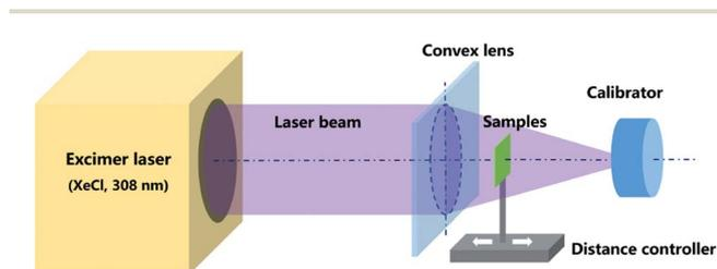
Fig. 1 Schematic depicting the ELA system applied to GZO films.
