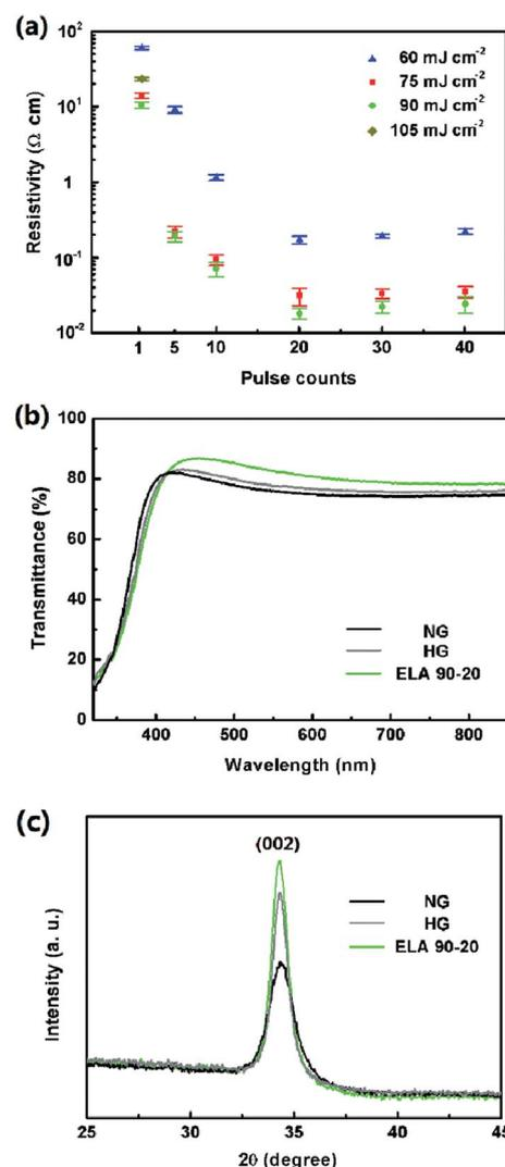
Fig. 2 (a) Variation of resistivity of ELA-treated GZO films with pulse counts (1, 5, 10, 20, and 40) under fluence at 60, 75, 90, and  $105 \text{ mJ cm}^{-2}$ . (b) Transmittance spectra and (c) XRD patterns of NG, HG, and ELA 90-20 on glass.
