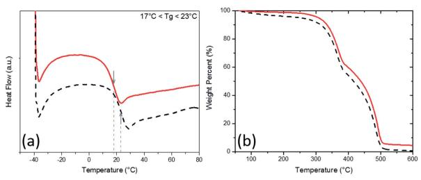
Fig. 4 (a) Differential scanning calorimetry and (b) thermogravimetric analysis of PU aerogels at bulk densities 0.28 g cm<sup>-3</sup> (solid line) and  $0.37 \text{ g cm}^{-3}$  (dash line).
