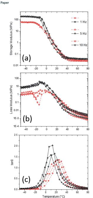
Fig. 7 Dynamic mechanical analysis in compression mode ((a): storage modulus, (b): loss modulus, and (c): tan delta) of PU aerogels at bulk densities 0.28 (dash line) and 0.37 (solid line) g  ${\rm cm}^{-3}$  at different temperatures and frequencies.
