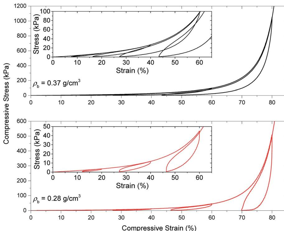
**Fig. 6** Quasi-static load-unload-reload compression testing of PU aerogels at bulk densities of 0.28 and 0.37 g cm<sup>-3</sup>.
