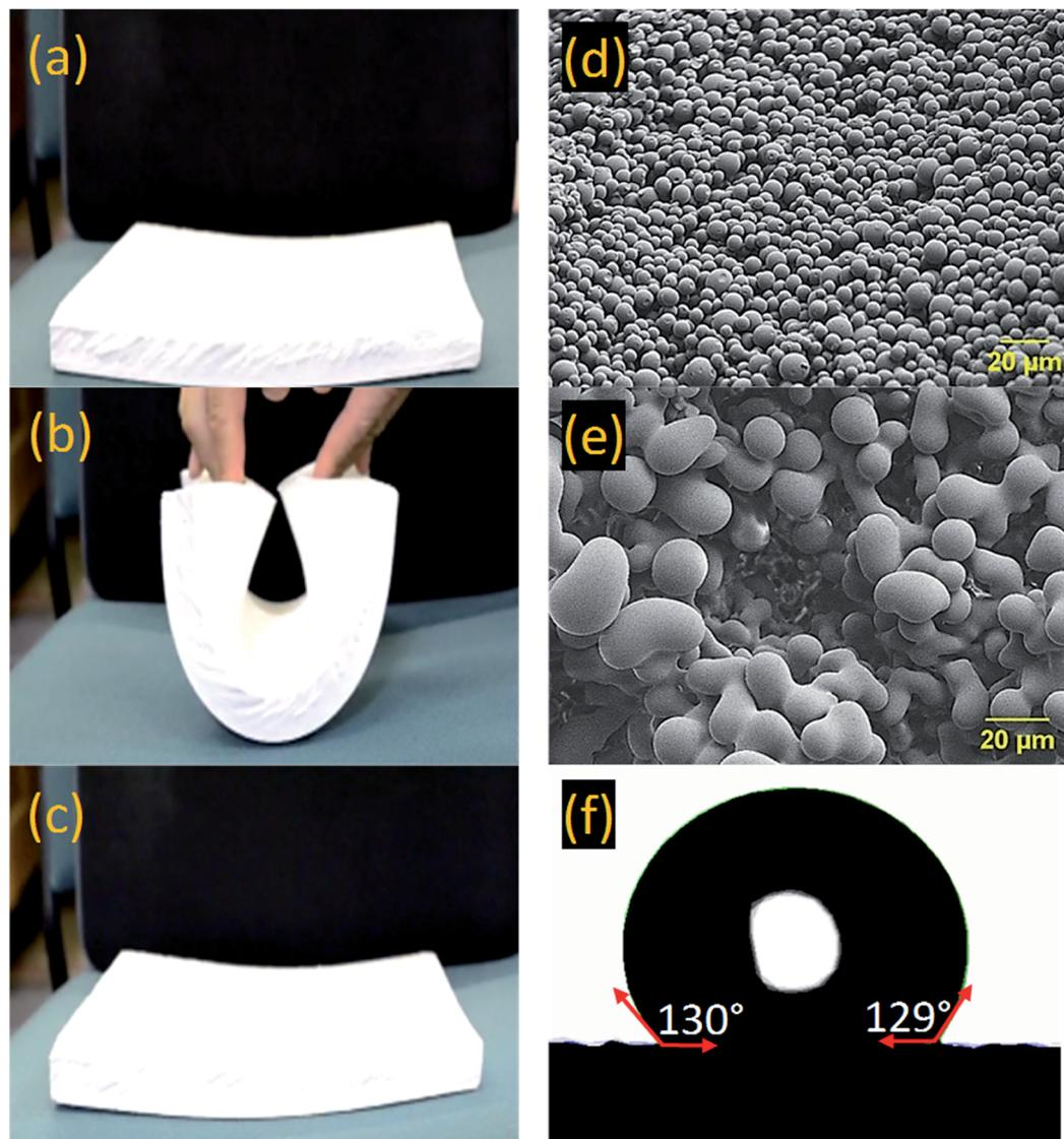
Fig. 3 Typical flexible PU aerogel panel at (a) original, (b) deformed and (c) final shapes at bulk density  $0.28 \text{ g cm}^{-3}$ ; (d) and (e) SEM images of the PU aerogels at bulk densities  $0.28 \text{ g cm}^{-3}$  and  $0.37 \text{ g cm}^{-3}$ , respectively; (f) water drop contact angles on the surface of the PU aerogel at bulk density  $0.28 \text{ g cm}^{-3}$ .
