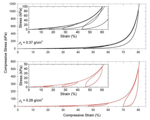
Quasi-static load-unload-reload compression testing of PU aerogels at bulk densities of 0.28 and 0.37 g cm<sup>-3</sup>.
