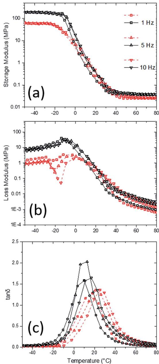
Fig. 7 Dynamic mechanical analysis in compression mode ((a): storage modulus, (b): loss modulus, and (c): tan delta) of PU aerogels at bulk densities 0.28 (dash line) and 0.37 (solid line)  $\text{g cm}^{-3}$  at different temperatures and frequencies.
