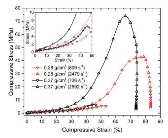
Fig. 8 Room temperature compressive behavior of PU aerogels at bulk densities 0.28 (dash line) and 0.37 (solid line) g  ${\rm cm}^{-3}$  at high strain rates.
