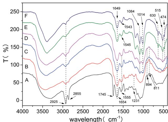
Fig. 7 FTIR spectra of different biomineralization periods (pH 2.5). Spectra A–F are at 12<sup>th</sup> hours and 1<sup>st</sup>, 2<sup>nd</sup>, 4<sup>th</sup>, 6<sup>th</sup>, 11<sup>th</sup> day, respectively.
