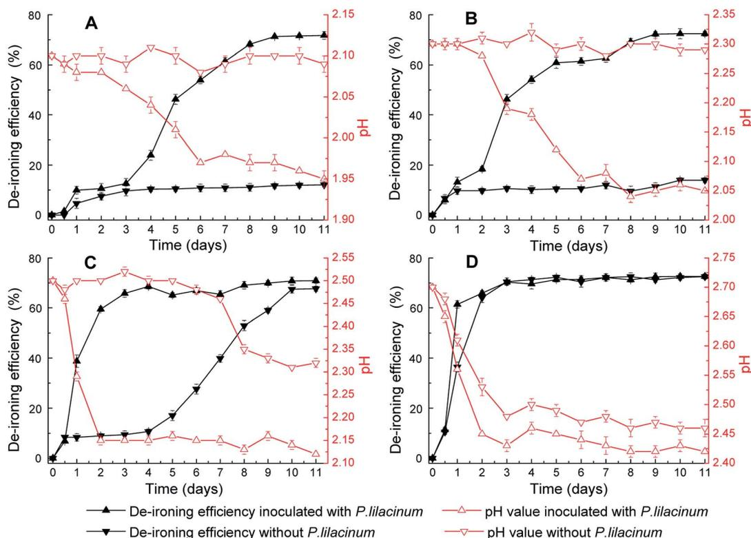
Fig. 2 The variation of setting efficiency of  $\text{Fe}^{3+}$  and pH value over time during biomineralization process induced *P. lilacinum* at different initial pH: (A) pH 2.1; (B) pH 2.3; (C) pH 2.5; (D) pH 2.7.
