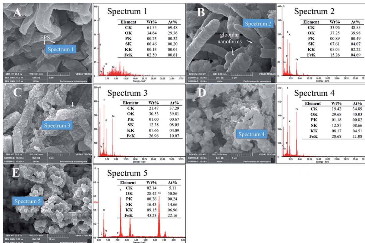
Fig. 4 SEM micrographs analysis showing the biomineralization process in different time (pH 2.5): (A) 12<sup>th</sup> hour; (B) 1<sup>st</sup> day; (C) 2<sup>nd</sup> day; (D) 11<sup>th</sup> day. And the precipitation of control experiments without cells: (E) 11<sup>th</sup> day.
