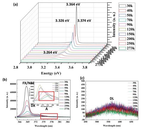
Fig. 7 LTPL spectra (a), ultraviolet (b) and visible (c) region spectra of Aq-ZnO nanowires with sputtering time of 120 s.
