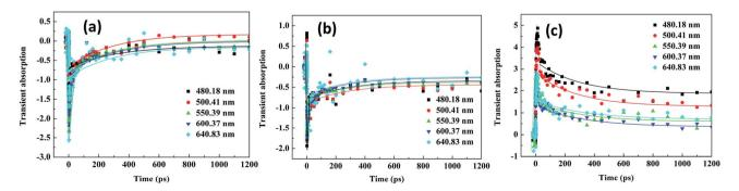
Fig. 11 Pump-probe transients of Ag-ZnO nanowires with sputtering time of 120 s excited at different wavelengths (325, 380 and 400 nm) and probed at different wavelengths.
