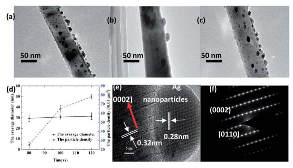
Fig. 4 TEM of Ag-ZnO nanowires with sputtering times of (a) 80 s, (b) 100 s, and (c) 120 s; (d) Average diameter and particle density of Ag-ZnO nanowires with sputtering times of 80 s, 100 s, and 120 s. HRTEM (e) and SAED image (f) of the Ag-ZnO nanowires for the sputtering time of 100 s.
