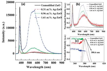
Fig. 6 PL (a) and normalized PL spectra (b and c) of unmodified ZnO and Aq-ZnO nanowires
