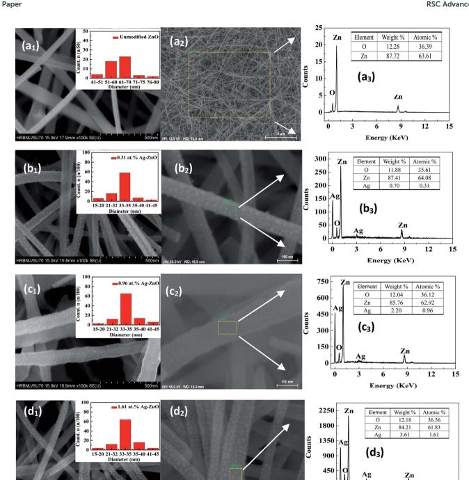
Fig. 2 Top-view SEM images (a1-d1), magnified SEM images (a2-d2), EDX spectra (a3-d3) for Ag-ZnO nanowires with sputtering times of 0 s, 80 s, 100 s, and 120 s, respectively.
