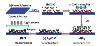
Scheme 1 Fabrication of the Ag-ZnO nanowires: (a) quartz substrate cleaned using the modified dip-coating method; (b) ZnO nanowires etched with Ar carrier gas; (c) as-deposited ZnO nanowires; (d) Ag nanoparticles produced for different sputtering times; (e) the Ag/ZnO nanostructure; (f) PL measurement.
