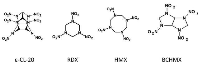
Fig. 1 Structural formulas of the studied cyclic nitramines.
