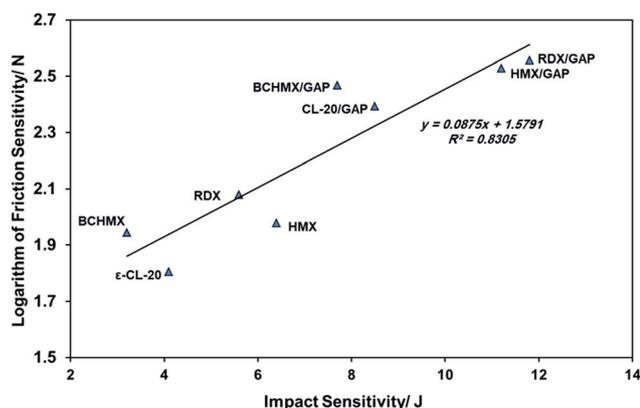
Fig. 2 Semi-logarithmic relationship between friction and impact sensitivities.
