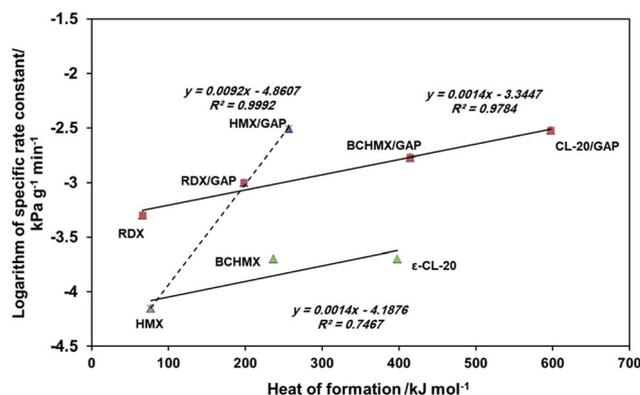
Fig. 6 Relationship between the logarithm of the specific rate constant and heat of formation of the studied PBXs and pure nitramines.
