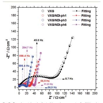
Fig. 7 Experimental and adjusted impedance spectra for lithium ion electro-insertion in VXG (black), VXG/NDI-ph1 (red), VXG/NDI-ph3 (blue) and VXG/NDI-ph1 (magenta) at 0.3 V.  $R_{\Omega}$  was subtracted for better comparison; these values are reported in Table 1.
