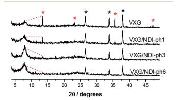
Fig. 6 XRD patterns of VXG and the VXG/NDI-ph (1, 3 and 6) intercalates ( $\lambda$  Cu K $\alpha$  = 1.54 Å) after 30 electrochemical cycles (cutoff *E* 4.47 V to 2.07 vs. Li/Li<sup>+</sup>, j = 0.2 mA). The red asterisks belong to the lithium-bearing phase, and the black asterisks belong to the fluorine-doped thin oxide of the electrodes.
