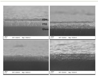
Fig. 4 Electron microscope images of the modified FTO electrodes, showing the composite layer regularity and adhesion to the electrode surface.
