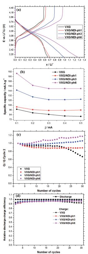
Fig. 5 (a) The amount of lithium ions inserted into the films as a function of the discharge/charge current from chronopotentiometry (cutoff E 4.47 V to 2.07 vs. Li/Li $^+$ , 0.2 mA) per mol of  $V_2O_5$ ; (b) the specific charge capacity at various current densities: (c) the discharge variation during 30 electrochemical cycles, compared to the second cycle  $(Q_n/Q_2, \text{ at 0.2 mA})$ ; (d) coulombic efficiency during 30 charge/ discharge cycles.
