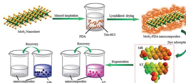
Fig. 1 Schematic illustration of the fabrication of MoS<sub>2</sub>-PDA composites by mussel-inspired chemistry.
