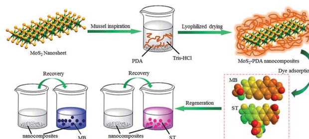
Fig. 1 Schematic illustration of the fabrication of MoS 2 -PDA composites by mussel-inspired chemistry.
