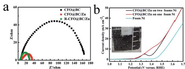
Fig. 4 (a) Electrochemical impedance spectra for R-CFO@BC/Zn, CFO@BC/Zn and CFO@BC at 1.55 V vs. RHE between 0.01 Hz to 100 000 Hz (b) LSV curves of CFO@BC/Zn on the Ni foam.
