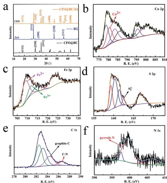
Fig. 1 (a) XRD patterns of CFO@BC/Zn hybrid and BG; (b), (c), (d), (e) and (f) high-resolution deconvoluted Co<sub>2p</sub>, Fe<sub>2p</sub>, S<sub>2p</sub>, C<sub>1s</sub> and N<sub>1s</sub> spectrum, respectively, of XPS data.
