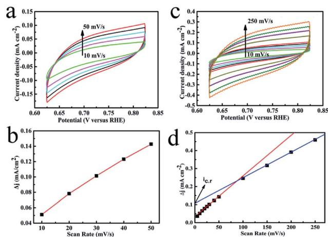
Fig. 5 (a) CV curves of CFO@BC/Zn from 10 to 50 mV s<sup>-1</sup>; (b) charging current density differences ( $\Delta j = j_a - j_c$ ) at 0.724 V vs. RHE; (c) CV curves of CFO@BC/Zn from 10 to 250 mV s<sup>-1</sup>; (d) dependence of the capacitive voltammetric current ( $\Delta j = j_a - j_c$ ) at 0.724 V vs. RHE.
