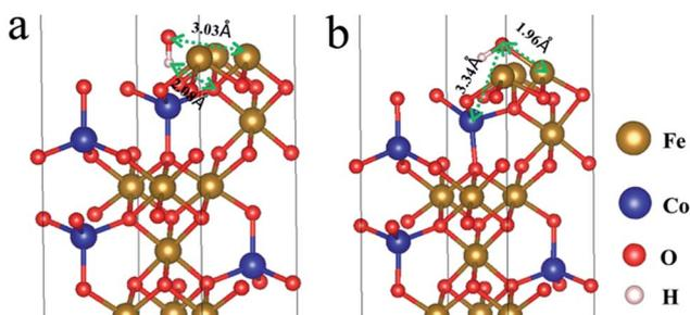
Fig. 6 (a) Adsorption of  $OH^-$  on the (100) surface of CFO before the system was optimized; (b) adsorption of  $OH^-$  on the (100) surface of CFO after the system was optimized.
