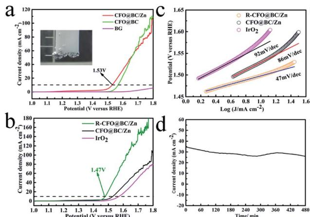
Fig. 3 (a) LSV curves of CFO@BC/Zn, CFO@BC and BG; (b) LSV curves of R-CFO@BC/Zn, CFO@BC/Zn and IrO<sub>2</sub>; (c) Tafel slopes of R-CFO@BC/Zn, CFO@BC and IrO<sub>2</sub>; (d) time dependence of the current density under a constant potential 1.53 V of CFO@BC/Zn hybrid.
