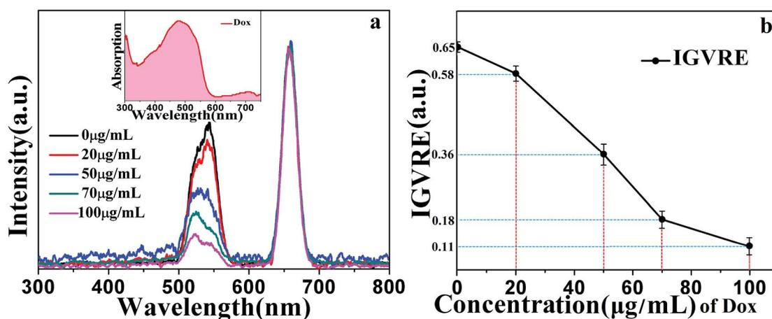
Fig. 5 (a) Room-temperature upconversion fluorescence spectra of  $NaGdF_4:18\% Yb^{3+}, 2\% Er^{3+}@NaYF_4$  core/shell particles with different concentrations of doxorubicin ( $0 \mu g mL^{-1}$ ,  $20 \mu g mL^{-1}$ ,  $50 \mu g mL^{-1}$ ,  $70 \mu g mL^{-1}$ , and  $100 \mu g mL^{-1}$ ) under the 980 nm excitation with power intensity of  $0.08 W cm^{-2}$  simultaneously. The inset shows the absorption spectrum of doxorubicin. (b) The ratio of simultaneous green and red emission intensity.
