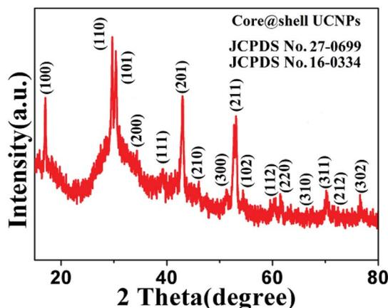
Fig. 3 XRD spectrum of  $\text{NaGdF}_4\text{:18% Yb}^{3+},\text{2%Er}^{3+}@NaYF_4$  core/shell particles.
