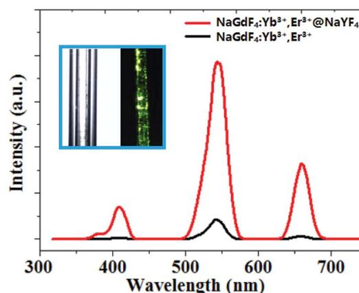
Fig. 4 Room temperature upconversion emission spectrum of core/shell  $\text{NaGdF}_4\text{:18% Yb}^{3+},\text{2%Er}^{3+}@NaYF_4$  and bare  $\text{NaGdF}_4\text{:18% Yb}^{3+},\text{2%Er}^{3+}$  nanoparticles. The inset: the photograph of core/shell UCNPs dispersed in CGT under the  $0.08\text{ W cm}^{-2}$  laser power at 980 nm excitation.
