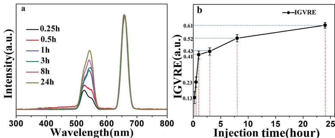
Fig. 6 (a) Evolution of the fluorescence intensity of core/shell UCNPs with the same concentration at different time points under 980 nm-excitation with power intensity of  $0.08 \text{ W cm}^{-2}$ . (b) The ratio of green and red emission intensity at the different time points.
