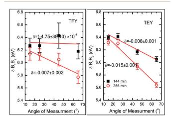
Fig. 6 Variation of  $B_2$  and  $B_1$  differences ( $\delta B_1 B_2$ ) with the angles of measurements for MgO sputtering durations of 144 and 256 min in both the TFY mode (left panel) and TEY mode (right panel), where  $\delta$  denotes the slope in eV per degree of the respective curve.
