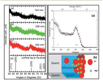
Fig. 7 X-ray diffraction pattern of sputtered MgO for durations of: (a) 144, (b) 256, and (c) 400 min along with a reference pattern corresponding to (d) JCPDS card no 78-0430 (left panel). Right panel shows: (a) experimental (symbol) and simulated (line) Rutherford backscattering (RBS) spectra for a sputtering duration of 400 min along with (b) a schematic of the model used for simulation.
