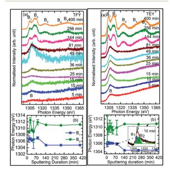
Fig. 4 (a) TFY- and (b) TEY-mode Mg K-edge NEXAFS spectra of sputtered MgO for different durations. In (b), the positions of the main spectral features B,  $B_1$ , and  $B_2$  are also shown for the measured spectra in the TFY mode (left panel) and TEY mode (right panel). Inset (b) (right panel), de-convolution of the spectral features
