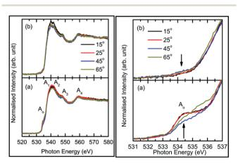
Fig. 10 O K-edge spectra of: (a) as-deposited and (b) annealed film for a sputtering duration of 400 min (left panel). Spectral features are mentioned as  $A_{\rm o}$ ,  $A_{\rm 1}$ ,  $A_{\rm 2}$ ,  $A_{\rm 3}$ , and  $A_{\rm 4}$ . Pre-regions at a zoomed-in scale for: (a) as-deposited and (b) annealed films are shown in the right panels.
