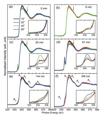
Fig. 3 TFY O K-edge spectra of MgO sputtered on quartz substrate at different angles (15°, 25°, 45°, and 65°) for deposition durations of: (a) 0 min, (b) 5 min, (c) 25 min, (d) 81 min, (e) 144 min, and (f) 256 min. The spectral features Ao, A1, A2, A3, and A4 are mentioned in panels in (e) and (f). The inset of each panel shows a zoomed-in section of the preedge region. Arrows highlight the shoulder in these spectra.
