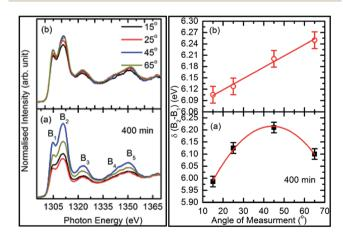
Fig. 11 Mg K-edge spectra for: (a) sputtering duration of 400 min and (b) annealed counterpart in TFY mode (left panel) for different angles of measurement ( $15^{\circ}$ ,  $25^{\circ}$ ,  $45^{\circ}$ , and  $60^{\circ}$ ). Spectral features of these spectra are denoted using  $B_1$ ,  $B_2$ ,  $B_3$ ,  $B_4$ , and  $B_5$ . Differences in the spectral features for: (a) sputtering duration of 400 min and (b) annealed counterpart with the angle are shown in the right panels.
