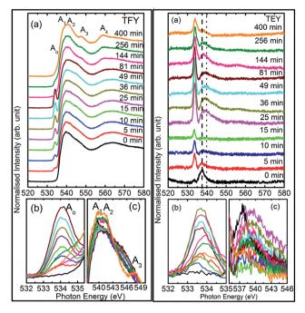
Fig. 2 Left panel shows (a) TFY O K-edge spectra of MgO sputtered on fused quartz substrate, (b) pre-edge spectral feature,  $A_{\text{o}}$ , and (c)  $A_{\text{1}}$ ,  $A_{\text{2}}$ ,  $A_{\text{3}}$  spectral feature regions right panel shows the corresponding measurements in TEY mode. Numerals in both panels represent the sputtering duration.
