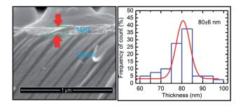
Fig. 8 Cross-sectional SEM image (left panel) and thickness profile (right panel) determined for a deposition time of 400 min.
