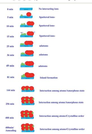
Fig. 12 Schematic of MgO growth for various sputtering durations and for the annealed counterpart of sputtering duration of 400 min.
