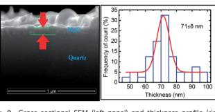
Fig. 9 Cross-sectional SEM (left panel) and thickness profile (right panel) for annealed sputtered species with a sputtering duration of 400 min
