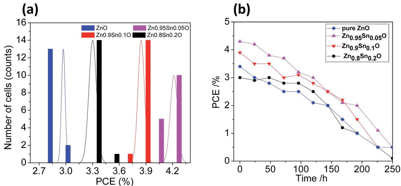
Fig. 7 (a) The PCE distribution histogram and (b) the PCE evolution of encapsulated devices stored in ambient air for different time periods [pure ZnO, Zn<sub>0.95</sub>Sn<sub>0.05</sub>O, Zn<sub>0.9</sub>Sn<sub>0.1</sub>O and Zn<sub>0.8</sub>Sn<sub>0.2</sub>O].
