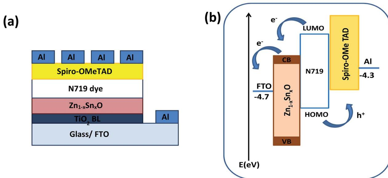
Fig. 1 (a) Schematic diagram and (b) energy level diagram of the FTO/TiO<sub>2</sub> BL/Zn<sub>1-x</sub>Sn<sub>x</sub>O/N719 dye/spiro-OMeTAD/Al device.
