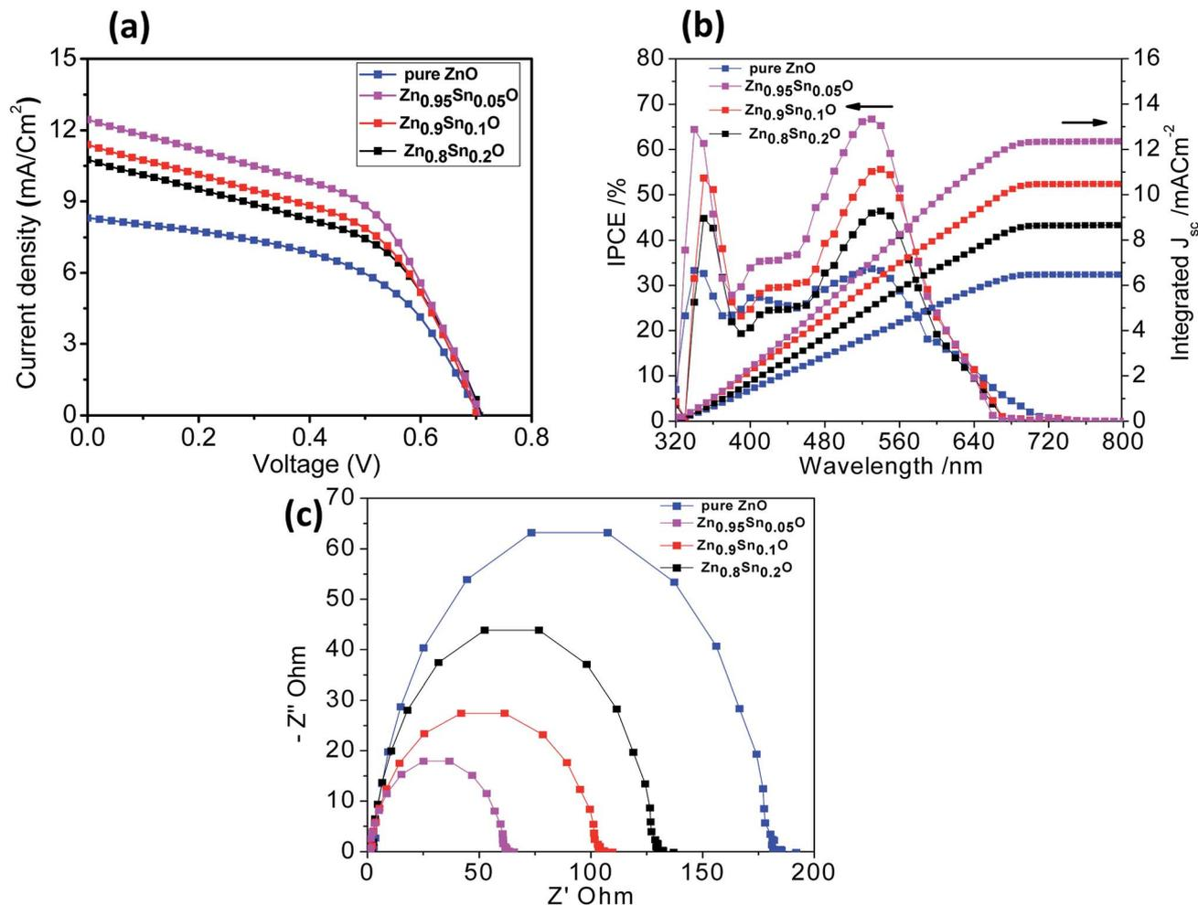
Fig. 6 (a)  $J$ - $V$  curves, (b) IPCE spectra and (c) Nyquist diagrams of the impedance spectra of pure ZnO, Zn<sub>0.95</sub>Sn<sub>0.05</sub>O, Zn<sub>0.9</sub>Sn<sub>0.1</sub>O and Zn<sub>0.8</sub>Sn<sub>0.2</sub>O.
