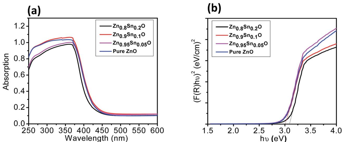
**Fig. 5** (a) UV-vis and (b) band gap of pure ZnO, Zn<sub>0.95</sub>Sn<sub>0.05</sub>O, Zn<sub>0.9</sub>Sn<sub>0.1</sub>O and Zn<sub>0.8</sub>Sn<sub>0.2</sub>O.
