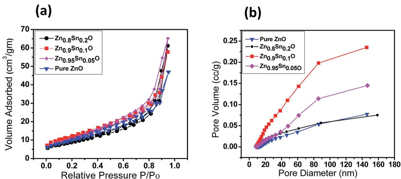
Fig. 4 (a) Nitrogen adsorption–desorption isotherms surface area and (b) pore size distribution of pure ZnO,  $\text{Zn}_{0.95}\text{Sn}_{0.05}\text{O}$ ,  $\text{Zn}_{0.9}\text{Sn}_{0.1}\text{O}$  and  $\text{Zn}_{0.8}\text{Sn}_{0.2}\text{O}$ .
