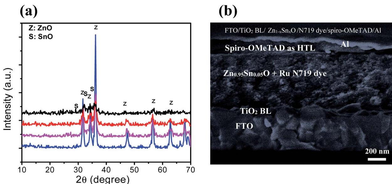
Fig. 2 (a) XRD spectra of pure ZnO (blue color), Zn<sub>0.95</sub>Sn<sub>0.05</sub>O (purple color), Zn<sub>0.9</sub>Sn<sub>0.1</sub>O (red color) and Zn<sub>0.8</sub>Sn<sub>0.2</sub>O (black color). (b) Cross sectional view of solid-state DSSCs containing a bi-oxide Zn<sub>0.95</sub>Sn<sub>0.05</sub>O photoelectrode.
