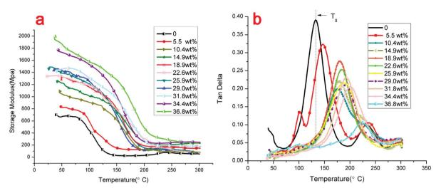
Fig. 7 Dynamic mechanical properties of novolac epoxy and modified GO/novolac epoxy composites: (a) storage modulus, (b) loss factor.
