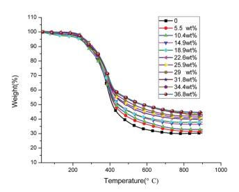
Fig. 5 TG curves of novolac epoxy and modified GO/novolac epoxy composite.
