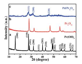
Fig. 1 XRD patterns of (a) Pr(OH)<sub>3</sub> precursor, (b) Pr<sub>6</sub>O<sub>11</sub> NRs and (c) Pd/ Pr<sub>6</sub>O<sub>11</sub> nanocatalysts (1.42 wt% Pd).
