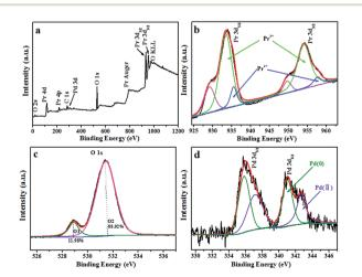
Fig. 3  $\,$  XPS analysis of Pd/Pr<sub>6</sub>O<sub>11</sub> samples (a) survey XPS spectrum, (b) Pr 3d; (c) O 1s and (d) Pd 3d.
