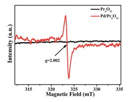
Fig. 4 The X-band EPR spectra of  $\rm Pr_6O_{11}$  and  $\rm Pd/Pr_6O_{11}$  samples recorded at 140 K.
