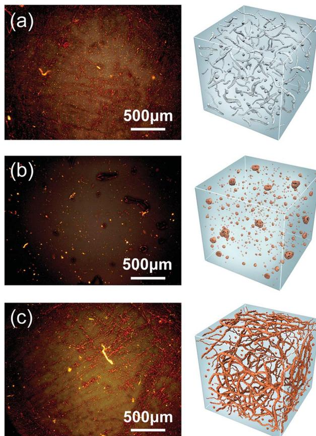
Fig. 3 Polarized optical microscope (POM) images for (a) BDO-PU, (b) monoFc-PU, and (c) bisFc-PU with 4× magnifications at 35 °C, as well as the corresponding illustration for superstructure consisted of the crystalline phases and amorphous phases.
