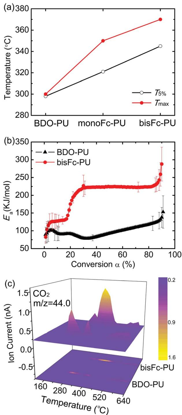
Fig. 1 (a) The initial degradation temperature ( $T_{5\%}$ ) and initial stage decomposition temperature ( $T_{max}$ ) of polyurethanes derived from the thermogravimetric analysis (TGA); (b) the comparison of activation energy ( $E_a$ ) for BDO-PU and bisFc-PU versus conversion  $\alpha$ ; (c) the thermogravimetry-quadrupole mass spectroscopy (TG-QMS) shows the release of  $CO_2$  during BDO-PU and bisFc-PU degradation from 100 to 775 °C.
