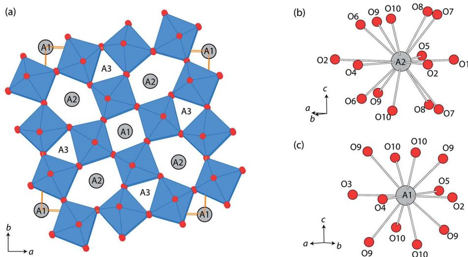
Fig. 1 (a) Crystal structure of tetragonal tungsten bronze projected along  $c$ -axis, and the coordination environments of (b) A2 and (c) A1 sites, using a particular example of  $\beta$ - $\text{SrTa}_2\text{O}_6$ .
