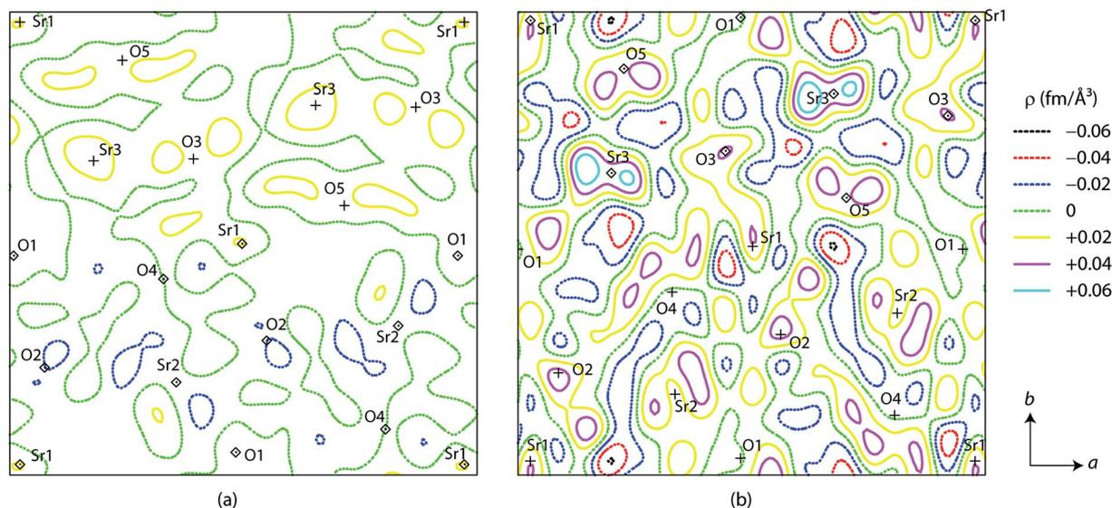
Fig. 6 Difference Fourier nuclear density for  $\text{Li}_x\text{Sr}_{1-0.5x}\text{Ta}_2\text{O}_6$ : (a)  $x = 0.08$  and (b)  $x = 0.17$ . Each contour diagram shows an area of  $13 \times 13 \text{ \AA}$  centered at  $(1/2, 1/2, 1/4)$  and perpendicular to  $c$ .
