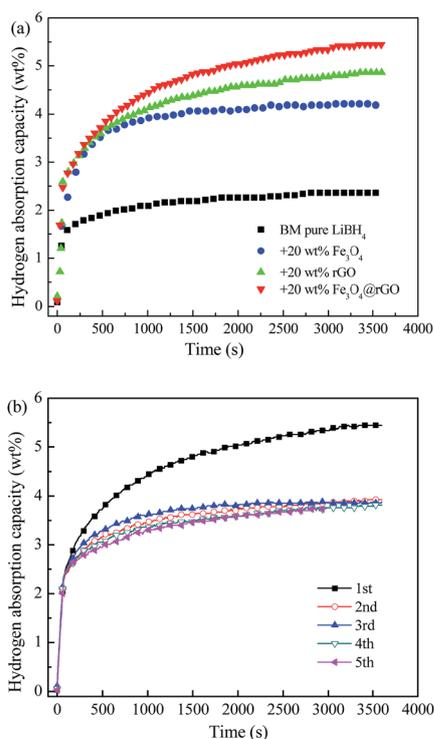
Fig. 6 (a) Isothermal rehydrogenation curves of the pure  $\text{LiBH}_4$  and  $\text{LiBH}_4$ -20 wt%  $y$  composites ( $y = \text{Fe}_3\text{O}_4$ , rGO, and  $\text{Fe}_3\text{O}_4$ @rGO), and (b) the rehydrogenation cycling stability of the  $\text{LiBH}_4$ -20 wt%  $\text{Fe}_3\text{O}_4$ @rGO composite at 400 °C under 5 MPa  $\text{H}_2$ .
