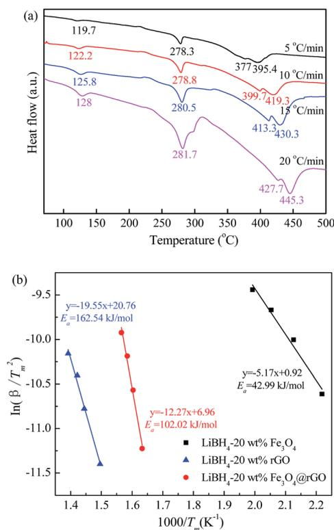
Fig. 4 (a) DSC curves for the LiBH<sub>4</sub>-20 wt% Fe<sub>3</sub>O<sub>4</sub>@rGO composite at various heating rates and (b) Kissinger's plots of  $E_a$  for the LiBH<sub>4</sub>-20 wt% y composites (y = Fe<sub>3</sub>O<sub>4</sub>, rGO, and Fe<sub>3</sub>O<sub>4</sub>@rGO).
