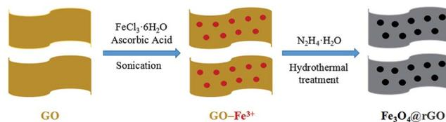
Scheme 1 Schematic illustration of the synthesis of the Fe<sub>3</sub>O<sub>4</sub>@rGO nanohybrid.
