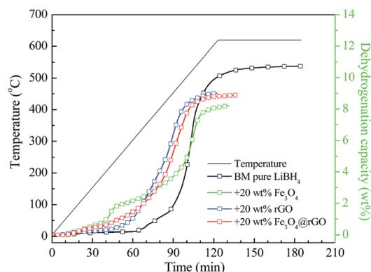
Fig. 3 TPD curves of ball-milled pure  $\text{LiBH}_4$ ,  $\text{LiBH}_4$ -20 wt%  $\text{Fe}_3\text{O}_4$ ,  $\text{LiBH}_4$ -20 wt% rGO, and  $\text{LiBH}_4$ -20 wt%  $\text{Fe}_3\text{O}_4$ @rGO composites.
