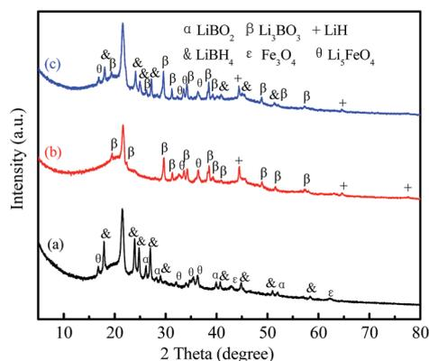
Fig. 8 XRD patterns of the  $\text{LiBH}_4\text{-20 wt% Fe}_3\text{O}_4\text{@rGO}$  composite: (a) as-milled, (b) after desorption at  $400^\circ\text{C}$ , and (c) after absorption at  $400^\circ\text{C}$ .
