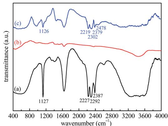
Fig. 9 FTIR spectra of the  $\text{LiBH}_4\text{-20 wt% Fe}_3\text{O}_4\text{@rGO}$  composite: (a) as-milled, (b) after desorption at  $400^\circ\text{C}$ , and (c) after absorption at  $400^\circ\text{C}$ .
