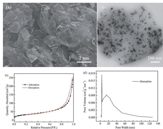
Fig. 1 (a) SEM image, (b) TEM image, (c) nitrogen adsorption–desorption isotherms, and (d) BJH pore-size distribution pattern of the as-prepared Fe<sub>3</sub>O<sub>4</sub>@rGO nanohybrid.
