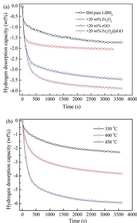
Fig. 5 Isothermal dehydrogenation curves of ball-milled (a) pure LiBH<sub>4</sub> and LiBH<sub>4</sub>-20 wt% y composites (y = Fe<sub>3</sub>O<sub>4</sub>, rGO, and Fe<sub>3</sub>O<sub>4</sub>@rGO) at 400 °C, and (b) the LiBH<sub>4</sub>-20 wt% Fe<sub>3</sub>O<sub>4</sub>@rGO composite at different temperatures.
