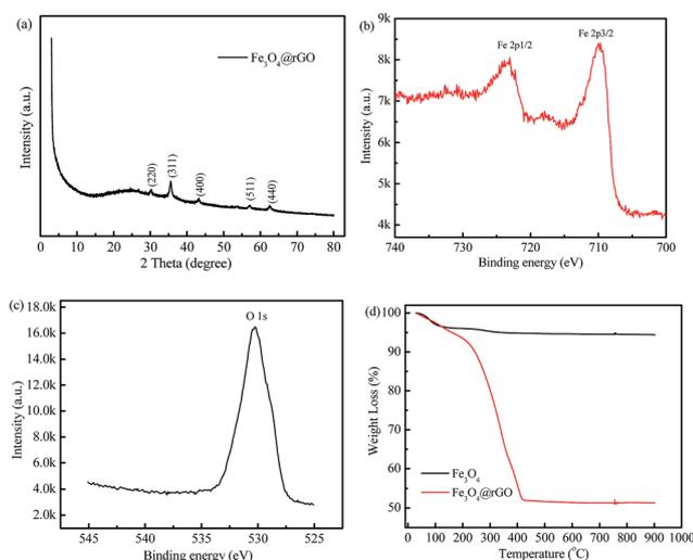
Fig. 2 (a) XRD pattern, (b) Fe 2p and (c) O 1s XPS spectra of the as-prepared  $\text{Fe}_3\text{O}_4$ @rGO nanohybrid, (d) TGA curves of  $\text{Fe}_3\text{O}_4$ @rGO and  $\text{Fe}_3\text{O}_4$  in air ranging from room temperature to 900 °C.
