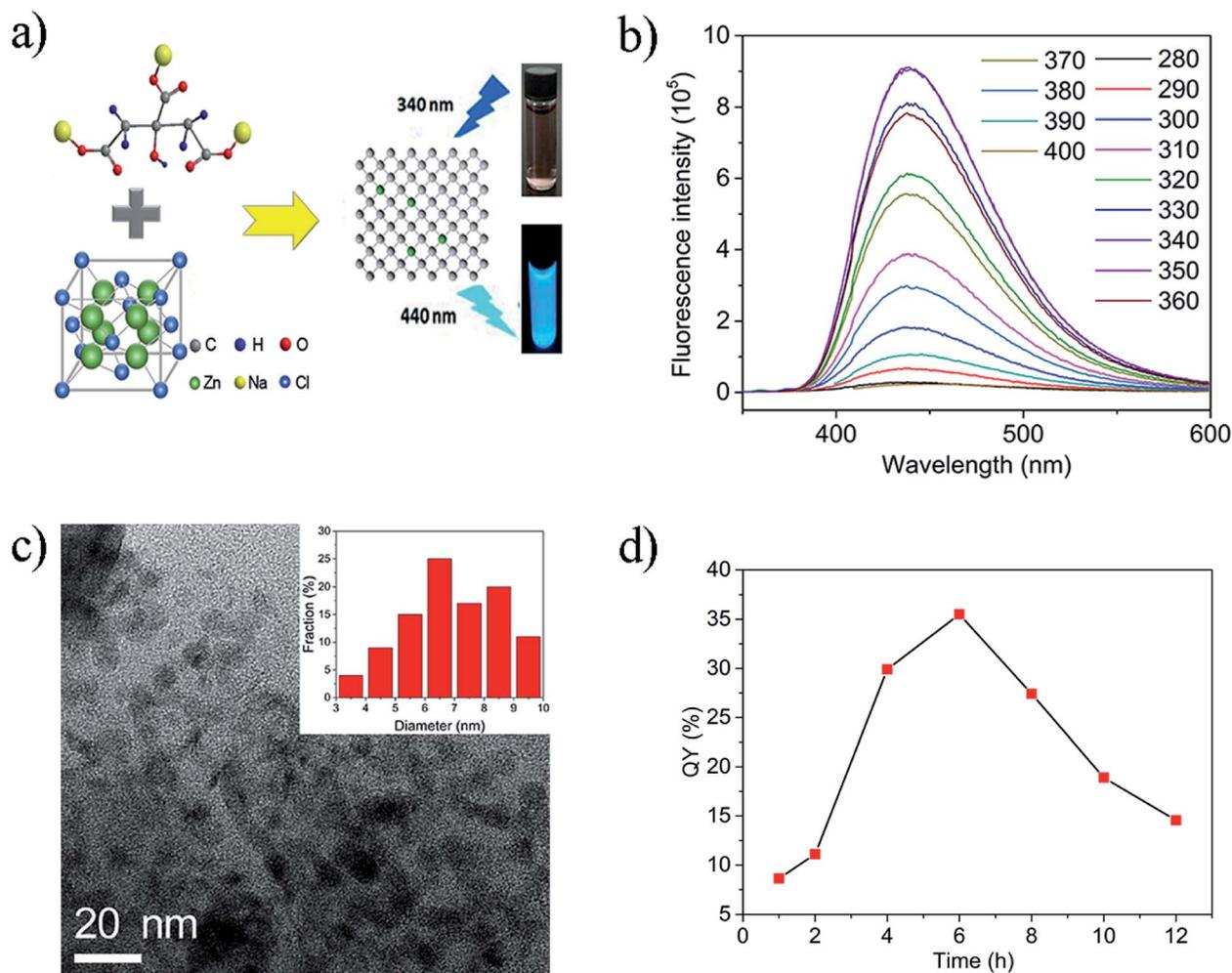
**Fig. 1** (a) Schematic diagram of the synthesis of the Zn-CDs with blue luminescence (excited by light at 340 nm); (b) photoluminescence spectra of the Zn-CDs; (c) TEM images of the Zn-CDs and the diameter distribution of the Zn-CDs; (d) quantum yield of the Zn-CDs for reaction times varying from 1 h to 12 h (1 h, 2 h, 4 h, 6 h, 8 h, 10 h, 12 h).
