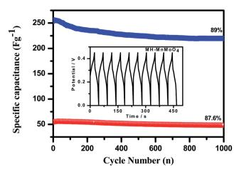
Fig. 11 Cycling performance of the Cp-MnMoO<sub>4</sub> and MH-MnMoO<sub>4</sub> electrodes at a current density of 5 A  $\rm g^{-1}$  (the inset figure shows the first ten galvanostatic charge–discharge profiles of the MH-MnMoO<sub>4</sub> electrode at 5 A  $\rm g^{-1}$ ).
