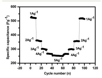
Fig. 12 Cycling stability test of the MH-MnMoO $_4$  electrode at various current densities for 100 cycles.
