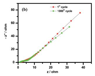
Fig. 13 Electrochemical impedance spectra of the (a) Cp-MnMoO<sub>4</sub> and (b) MH-MnMoO<sub>4</sub> electrodes after the  $1^{st}$  and  $1000^{th}$  galvanostatic charge–discharge cycles at a current density of 5 A  $\rm g^{-1}$ .
