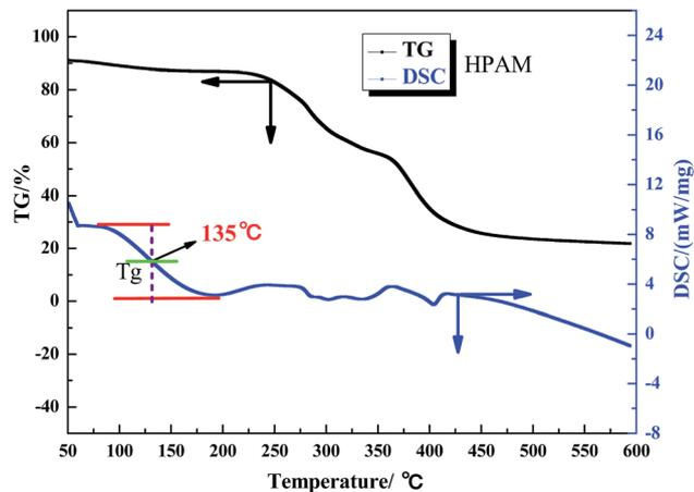
Fig. 5 TGA and DSC results for HPAM.
