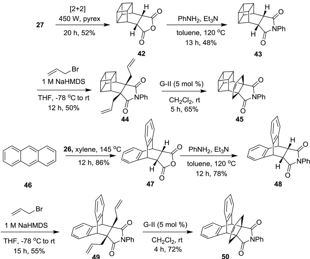
Scheme 6 Synthesis of the basketene-based and anthracene derived propellane derivatives **45** and **50**, respectively.
