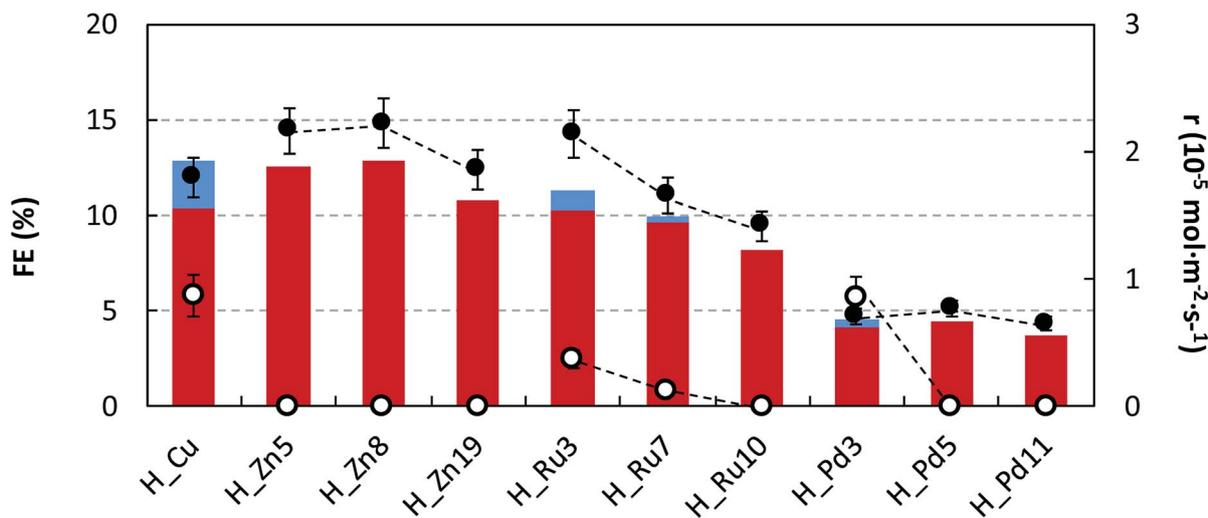
Fig. 7 FEs for  $C_2H_5OH$  (in red) and  $CH_3OH$  (in blue) formation and  $r$  for  $C_2H_5OH$  (●) and  $CH_3OH$  (○) in the electrocatalytic reduction of  $CO_2$  at H\_Zn, H\_Ru and H\_Pd in comparison to H\_Cu.
