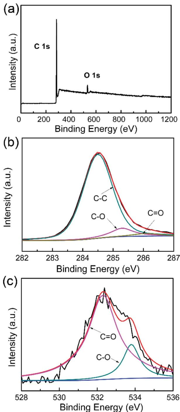
Fig. 3 (a) XPS survey spectra of WCNWs. (b and c) High resolution XPS spectra of (b) C 1s and (c) O 1s.
