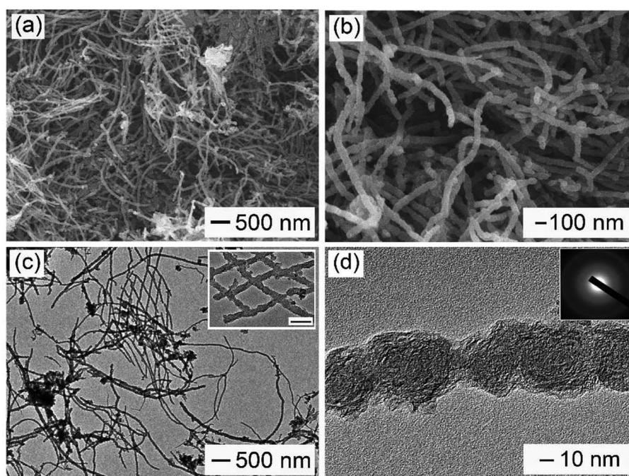
Fig. 1 (a) Low- and (b) high-magnification SEM images of WCNWs. (c) TEM and (d) high-resolution TEM images of WCNWs. The scale bar in the inset of part (c) is 100 nm, and the inset of part (d) is the selected-area electron diffraction (SAED) pattern of the WCNWs.
