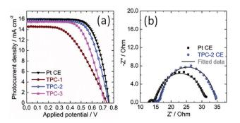
Fig. 6 (a) Characteristic photocurrent density–voltage curves of the DSCs with TPC CEs of different thicknesses and Pt CE, measured under solar simulator illumination of 100 mW cm<sup>-2</sup> (AM 1.5G); (b) electrochemical impedance spectra of DSCs using TPC-2 and Pt CEs measured under light irradiation, at open-circuit voltage; dots present experimental results, and solid lines show fitted results.
