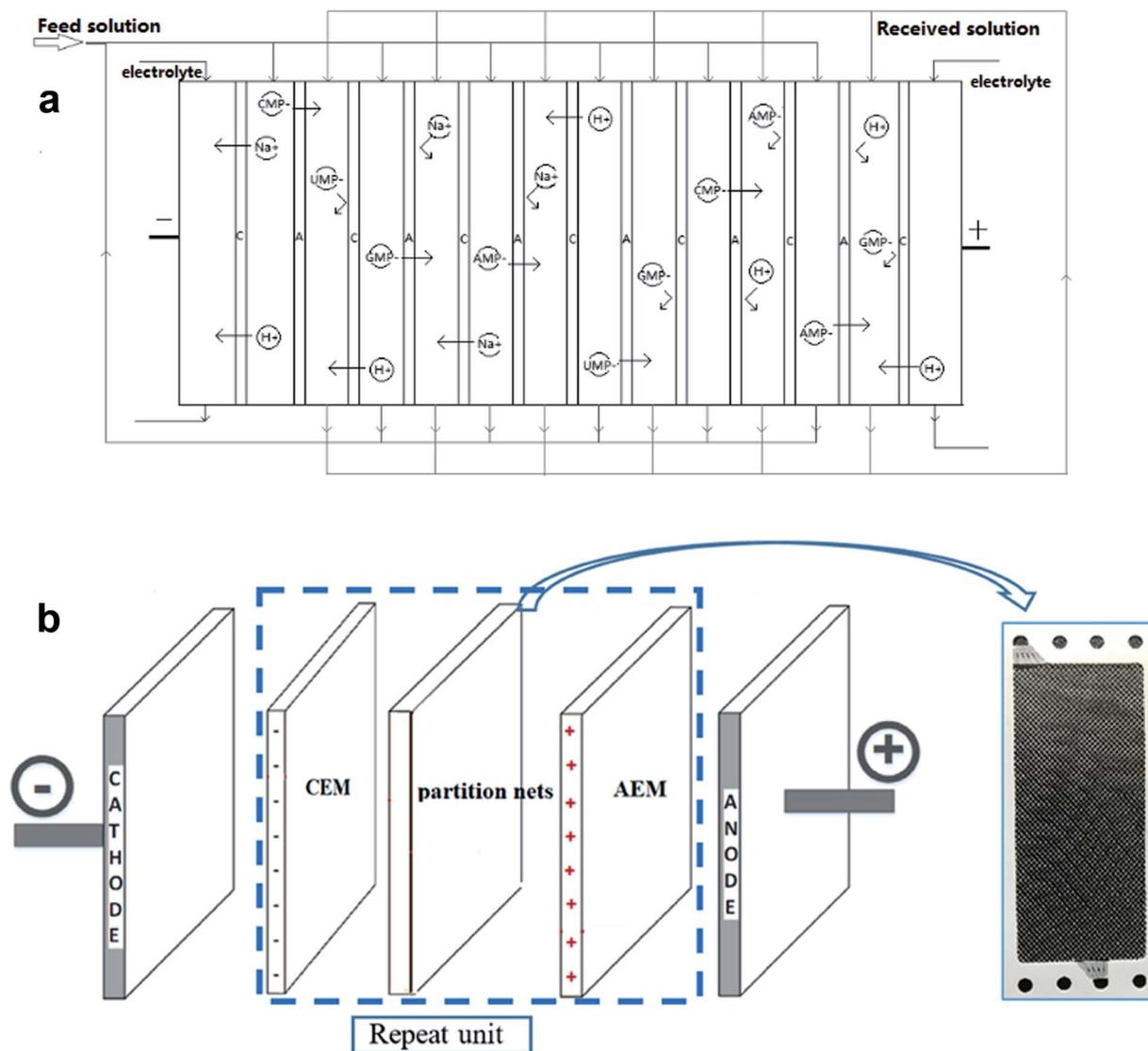
Fig. 2 (a) Principle of electrodiolysis to produce 5'-ribonucleotides. (b) Schematic diagram of the membrane stack.
