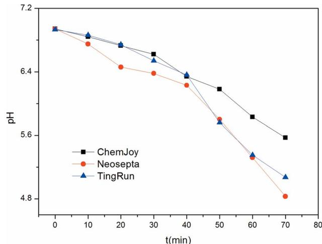
Fig. 5 pH trend in the feed compartment in the constant current operation.
