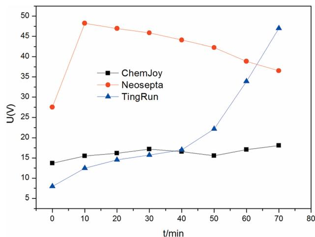
Fig. 4 Voltage trend of three different membranes in the case of  $I = 0.25$  A in the constant current operation.
