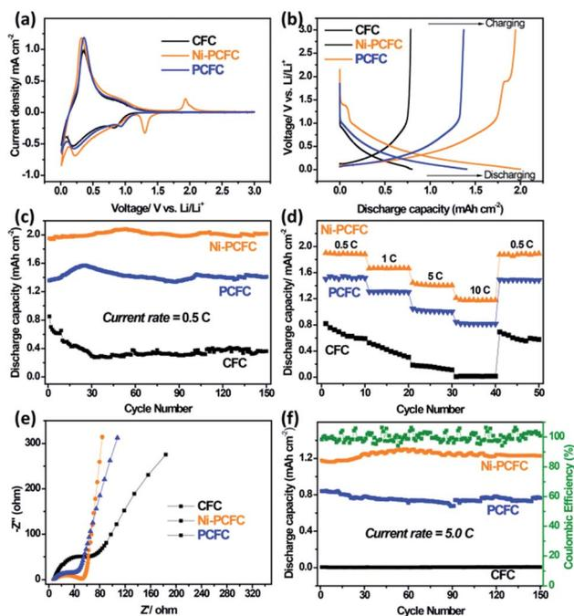
Fig. 4 (a) 3<sup>rd</sup> CV profile and (b) 3<sup>rd</sup> charge/discharge profile of CFC, Ni-PCFC and PCFC electrodes. (c) Cyclic stability at 0.5C, (d) Nyquist plots, (e) rate capability and (f) cyclic stability at 5C of the CFC, Ni-PCFC and PCFC anodes.
