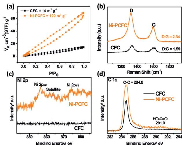
Fig. 3 (a) BET surface areas of CFC and Ni-PCFC. (b) Raman spectra, (c) Ni 2p XPS spectra and (d) C 1s XPS spectra of CFC and Ni-PCFC.
