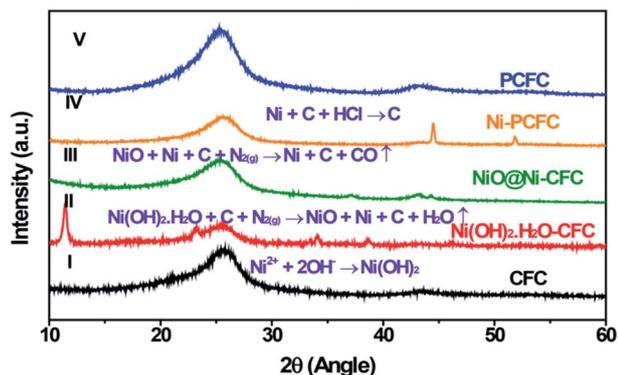
Fig. 1 XRD patterns showing the formation of Ni-PCFC and other samples. (I) CFC, (II) Ni(OH)<sub>2</sub>·H<sub>2</sub>O-CFC, (III) NiO@Ni-CFC, (IV) Ni-PCFC and (V) PCFC.
