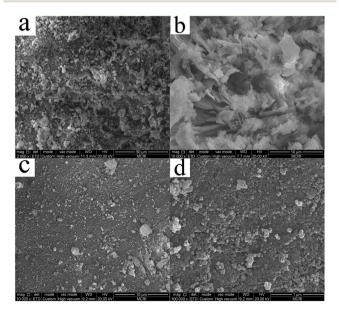
Fig. 10 SEM images of T600 before and after phosphate adsorption: (a) before adsorption  $\times 2000$ ; (b) before adsorption  $\times 10000$ ; (c) after adsorption  $\times 10000$ ; (d) after adsorption  $\times 10000$ .
