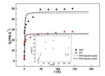
Fig. 2 Adsorption kinetics of phosphate removal on T600 at 4 and 20  $^{\circ}\text{C}.$
