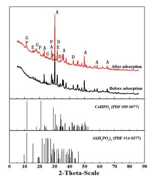
Fig. 9 XRD patterns of T600 before and after phosphate adsorption (A  $- Ca_2Al_2SiO_7$ ; D  $- Ca_3Al_2O_6 \cdot 6H_2O$ ; E  $- Ca_{12}Al_{14}O_{33}$ ; F  $- CaHPO_4$ ; G  $- Al(H_2PO_4)_3$ ).
