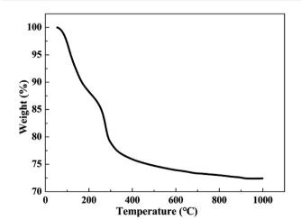
Fig. 1 TGA curve of HAC.
