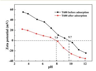
Fig. 7 Zeta potential of T600 before and after phosphate adsorption.
