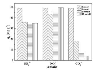
Fig. 5 Effect of coexisting anions on phosphate adsorption by T600.
