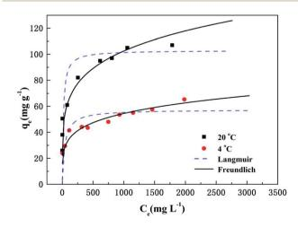
Fig. 3 Adsorption isotherms and models of phosphate removal on T600.
