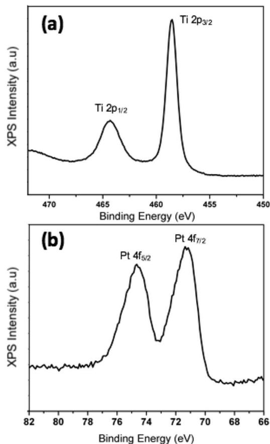
Fig. 6 XPS spectra of the Pt core and Ti shell after extended air exposure, nanoparticle mass 90 kDa. (a) Spectrum of Ti 2p doublet demonstrating the chemical state of  $\text{TiO}_2$  after full oxidation and (b) spectrum of Pt 4f doublet.
