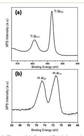
Fig. 6 XPS spectra of the Pt core and Ti shell after extended air exposure, nanoparticle mass 90 kDa. (a) Spectrum of Ti 2p doublet demonstrating the chemical state of  $\rm TiO_2$  after full oxidation and (b) spectrum of Pt 4f doublet.
