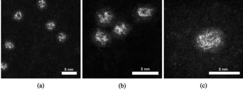
Fig. 2 90 kDa Pt-Ti nanoparticles prior to prolonged exposure to ambient conditions. It can be seen that the Pt is dispersed throughout the nanoparticle instead of forming a Pt core morphology. (a) and (b) Present lower magnification images. Left to right shows increasing magnification. The higher magnification image, (c), shows the amorphous structure in greater detail.
