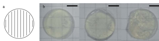
Fig. 3 (a) Illustration of the scan path for a cycloidal pattern (the red line represents the hatch distance), (b) photos of the green parts (cylinder with diameters of 14 mm and thicknesses of 1.4 mm) fabricated under different SL parameters (from left to right, 60 mW 46 mm \text{s}^{-1} , 130 mW 100 mm \text{s}^{-1} and 200 mW 154 mm \text{s}^{-1} , scale bar, 2.5 mm).
