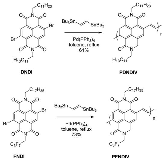
Scheme 1 Synthesis of PDNDIV and PFNDIV by Stille coupling reaction.
