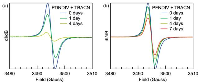
Fig. 4 Room-temperature X-band EPR spectra of (a) 2 mM (repeating units) PDNDIV with 10 mM TBACN and (b) 2 mM PFNDIV with 2 mM TBACN in THF yielding  $[\text{PDNDIV}]^{\cdot-}$  and  $[\text{PFNDIV}]^{\cdot-}$ , respectively. The 7 day point for  $[\text{PDNDIV}]^{\cdot-}$  is omitted and unreliable due to polymer precipitation.
