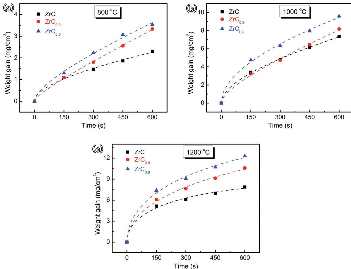
Fig. 14 Change in mass per unit surface area of ZrC<sub>1-x</sub> ceramic as a function of time for isothermal corrosion experiments at (a) 800 °C, (b) 1000 °C, and (c) 1200 °C, respectively.
