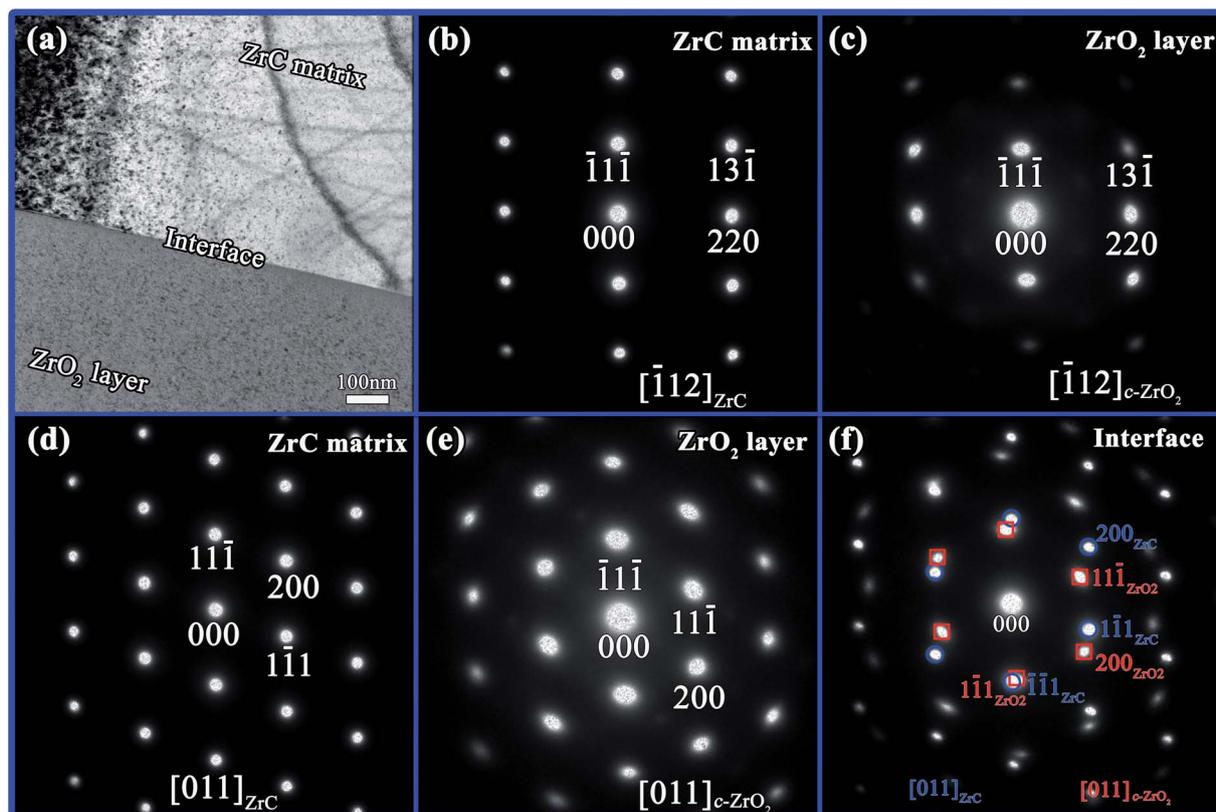
Fig. 9 (a) Bright-field TEM image of the matrix and corrosion layer corroded at 800 °C for 600 s, SAED patterns of (b) ZrC matrix and (c) ZrO<sub>2</sub> layer obtained from zone axis  $[\bar{1}12]$ , and SAED patterns of (d) ZrC matrix, (e) ZrO<sub>2</sub> layer, and (f) interface obtained from zone axis  $[011]$ .
