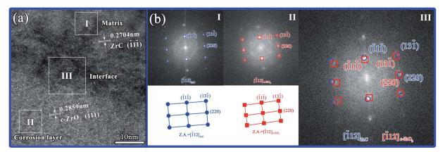
Fig. 11 (a) HR-TEM image of the interface of matrix and corrosion layer and (b) corresponding FFT images obtained from zone axis [112].
