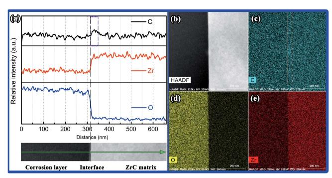
Fig. 12 (a) STEM-EDS line scan and element map of the interface of matrix and corrosion layer, (b) HADDF image, (c-e) C, O, and Zr element maps, respectively.
