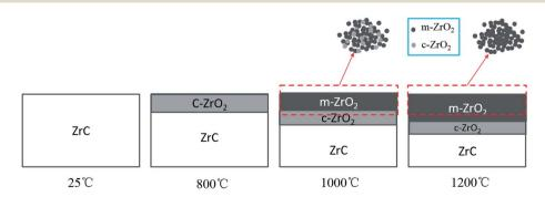
Fig. 3 Schematic of the oxide layer structure of ZrC ceramics after corrosion in water vapor at different temperatures, according to XRD pattern results from residual ceramics and spalled powders.
