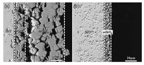
Fig. 7 Cross-section morphologies of (a) the unspalled corrosion layer and (b) residual layer after spallation of oxide layer from ZrC ceramics corroded at  $1000 \,^{\circ}$ C for  $600 \, s$ .
