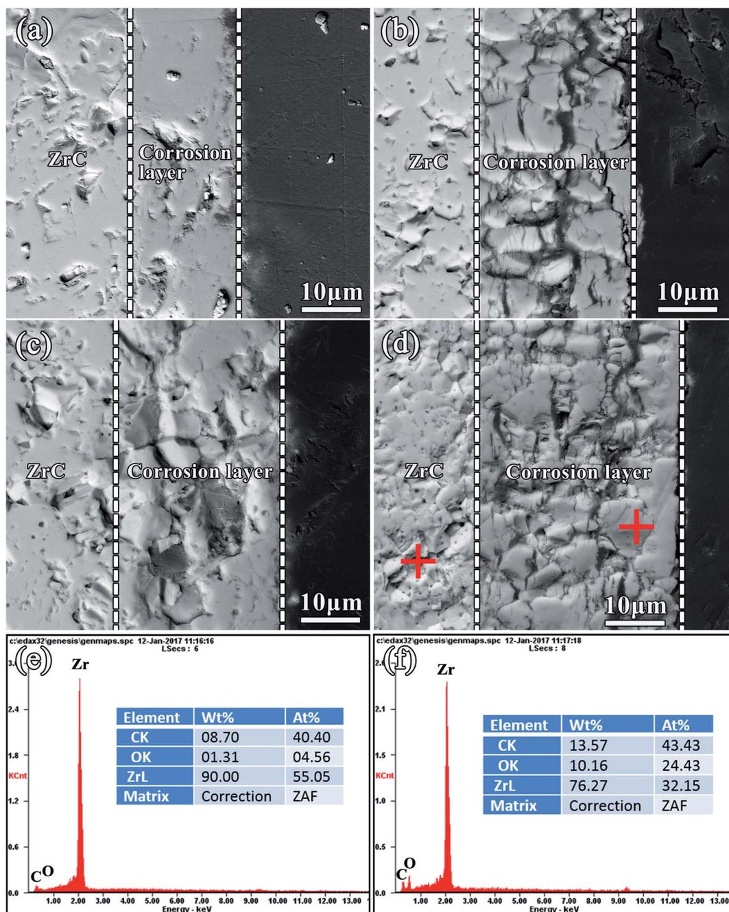
Fig. 6 Cross-section morphologies of corrosion layers for ZrC corroded at 800 °C for different times: (a–d) 150, 300, 450, and 600 s, respectively, and EDS spectra taken from (e) ZrC and (f) the corrosion layer.
