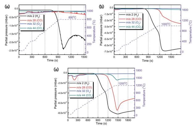
Fig. 4 Mass spectrographics of ZrC ceramics in water vapor during heating from RT to (a) 800 °C, (b) 1000 °C and (c) 1200 °C, respectively.
