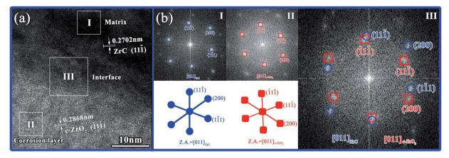
Fig. 10 (a) HR-TEM image of the interface of matrix and corrosion layer and (b) corresponding FFT images obtained from zone axis [011].
