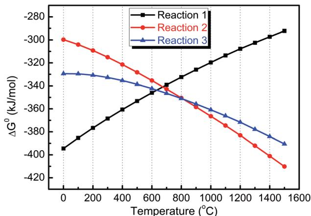
Fig. 5 Variation in  $\Delta G^0$  of different corrosion reactions as a function of temperature.
