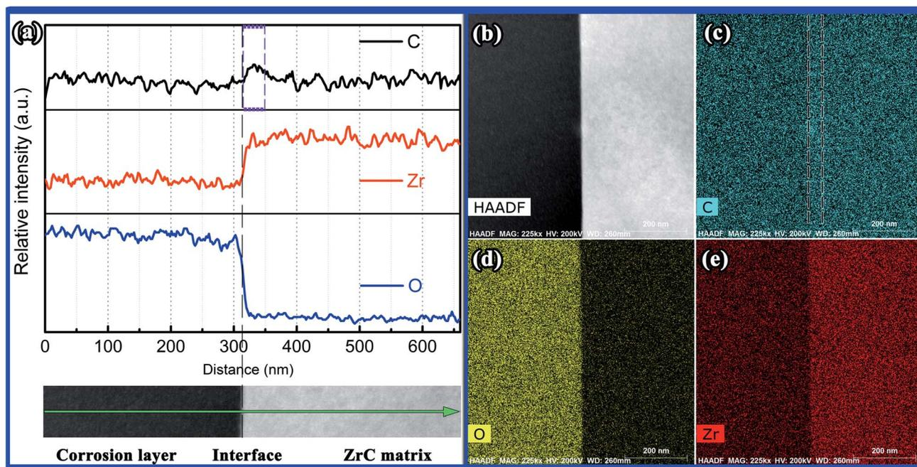
Fig. 12 (a) STEM-EDS line scan and element map of the interface of matrix and corrosion layer, (b) HAADF image, (c–e) C, O, and Zr element maps, respectively.
