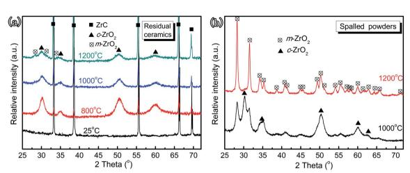
Fig. 2 XRD patterns of the ZrC ceramics pristine and corroded at 800–1200 °C after 600 s. Residual ceramics (a) and spalled powders (b).
