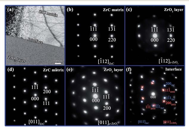
Fig. 9 (a) Bright-field TEM image of the matrix and corrosion layer corroded at 800 °C for 600 s, SAED patterns of (b) ZrC matrix and (c) ZrO<sub>2</sub> layer obtained from zone axis [112], and SAED patterns of (d) ZrC matrix, (e) ZrO<sub>2</sub> layer, and (f) interface obtained from zone axis [011].
