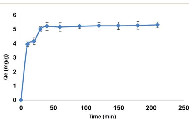
Fig. 10 Effect of extraction time on the adsorption capacity ( $q_t$ ) of LEV onto  $\text{Fe}_3\text{O}_4\text{@MIP}$  NPs; adsorbent:  $150 \text{ mg}$ , drug conc.  $100 \text{ mg L}^{-1}$ , temperature:  $25 \text{ }^\circ\text{C}$ , pH: natural pH of LEV, time: 210 min.
