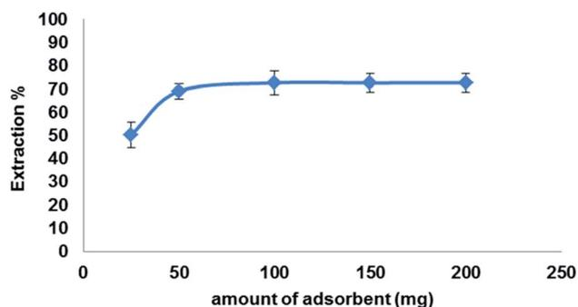
Fig. 12 Effect of adsorbent amount on the extraction efficiency of LEV onto  $\text{Fe}_3\text{O}_4$ @MIP NPs; drug conc.  $100 \text{ mg L}^{-1}$ , temperature:  $25^\circ\text{C}$ , pH: 7.0, time: 30 min.
