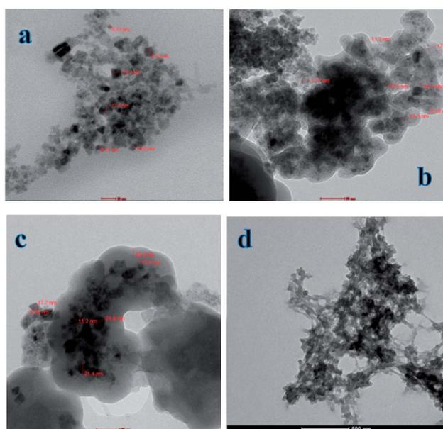
Fig. 3 TEM images of: [a]  $\text{Fe}_3\text{O}_4\text{@OA}$  NPs, [b]  $\text{Fe}_3\text{O}_4\text{@SiO}_2$  NPs, [c]  $\text{Fe}_3\text{O}_4\text{@MPS}$  NPs and [d]  $\text{Fe}_3\text{O}_4\text{@MIP}$  NPs.
