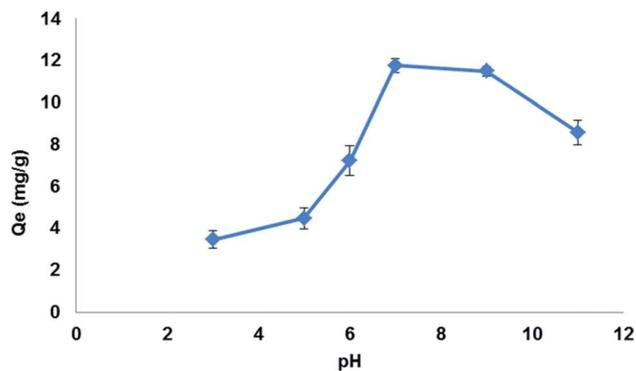
Fig. 11 Effect of pH on the adsorption capacity ( $q_e$ ) of LEV onto  $\text{Fe}_3\text{O}_4$ @MIP NPs. Adsorbent: 25 mg, drug conc.  $100 \text{ mg L}^{-1}$ , temperature:  $25^\circ\text{C}$ , time: 30 min.
