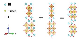
Fig. 1 Schematic representation of the crystalline structure of Bi $_3$ -TiNbO $_9$ -Bi $_4$ Ti $_3$ O $_{12}$ .
