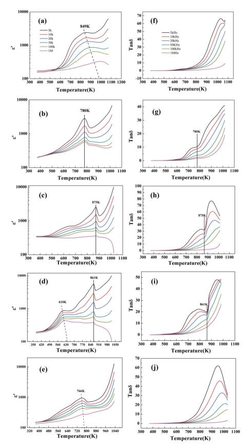
Fig. 8 Temperature dependency of dielectric constant ( $\varepsilon'$ ) and dielectric loss factor (tan  $\delta$ ) at 5 kHz-1 MHz of (a) and (f) BTN-2; (b) and (g) BLTNF-2.5; (c) and (h) BLTNF-3; (d) and (i) BLTNF-3.5; and (e) and (j) BTF-4 samples.
