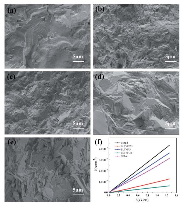
SEM micrographs of (a) BTN-2; (b) BLTNF-2.5; (c) BLTNF-3; (d) BLTNF-3.5; (e) BTF-4; (f)The J-E curve of the samples.
