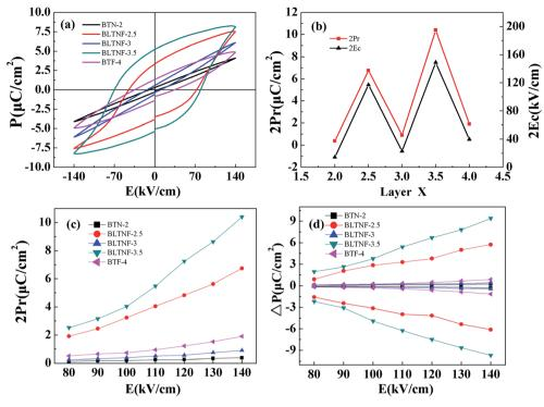
Fig. 7 (a) P-E hysteresis loops of the samples at 140 kV cm<sup>-1</sup> in 50 Hz; (b) dependence of  $2E_c$  and  $2P_r$  on the number of layer (x); and  $2P_r$  (c) and  $\Delta P$  (d) of the samples measured at different electrical field.
