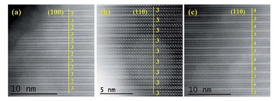
Fig. 3 STEM-HAADF images of (a)  $Bi_3TiNbO_9-Bi_3LaTiNbFeO_{12}$  (BLTNF-2.5); (b)  $Bi_3LaTiNbFeO_{12}$  (BLTNF-3); and (c)  $Bi_3LaTiNbFeO_{12}-Bi_5Ti_3FeO_{15}$  (BLTNF-3.5).
