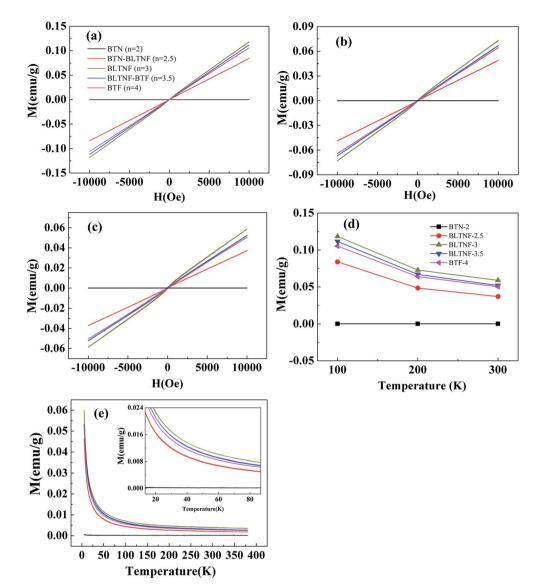
Fig. 9 The magnetic hysteresis loops of the samples measured at (a) 100 K; (b) 200 K; (c) 300 K; (d) dependence of magnetic polarization measured at 10 000 Oe and different temperatures; and (e) temperature dependence of magnetization of the samples in the ZFC-FC modes measured at 500 Oe.
