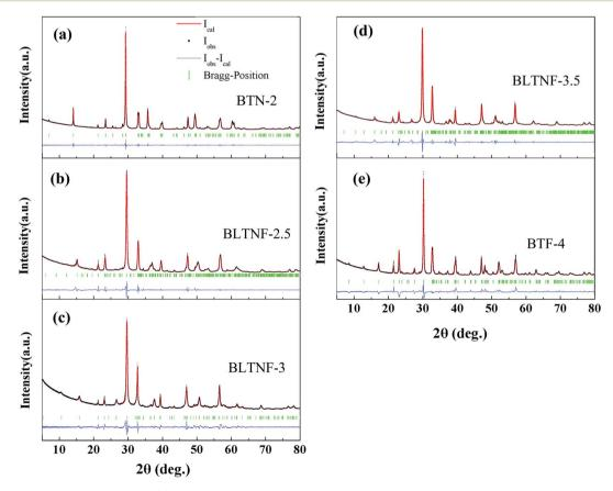
Fig. 2 XRD patterns and refined results of (a)  $Bi_3TiNbO_9$  (BTN-2); (b)  $Bi_3TiNbO_9 - Bi_3LaTiNbFeO_{12}$  (BLTNF-2.5); (c)  $Bi_3LaTiNbFeO_{12}$  (BLTNF-3); (d)  $Bi_3LaTiNbFeO_{12} - Bi_5Ti_3FeO_{15}$  (BLTNF-3.5); and (e)  $Bi_5Ti_3FeO_{15}$  (BTF-4).
