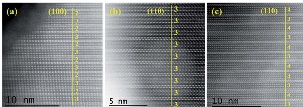
Fig. 3 STEM-HAADF images of (a)  $\text{Bi}_3\text{TiNbO}_9\text{-Bi}_3\text{LaTiNbFeO}_{12}$  (BLTNF-2.5); (b)  $\text{Bi}_3\text{LaTiNbFeO}_{12}$  (BLTNF-3); and (c)  $\text{Bi}_3\text{LaTiNbFeO}_{12}\text{-Bi}_5\text{Ti}_3\text{FeO}_{15}$  (BLTNF-3.5).
