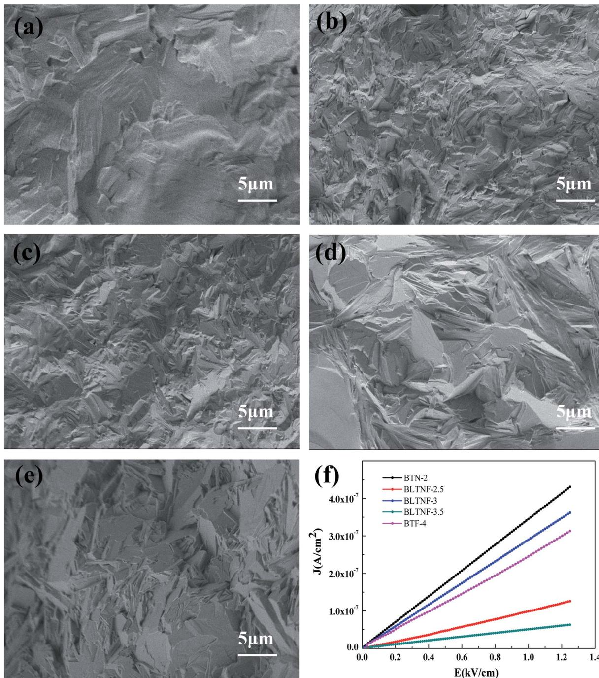
Fig. 6 SEM micrographs of (a) BTN-2; (b) BLTNF-2.5; (c) BLTNF-3; (d) BLTNF-3.5; (e) BTF-4; (f) The  $J$ - $E$  curve of the samples.
