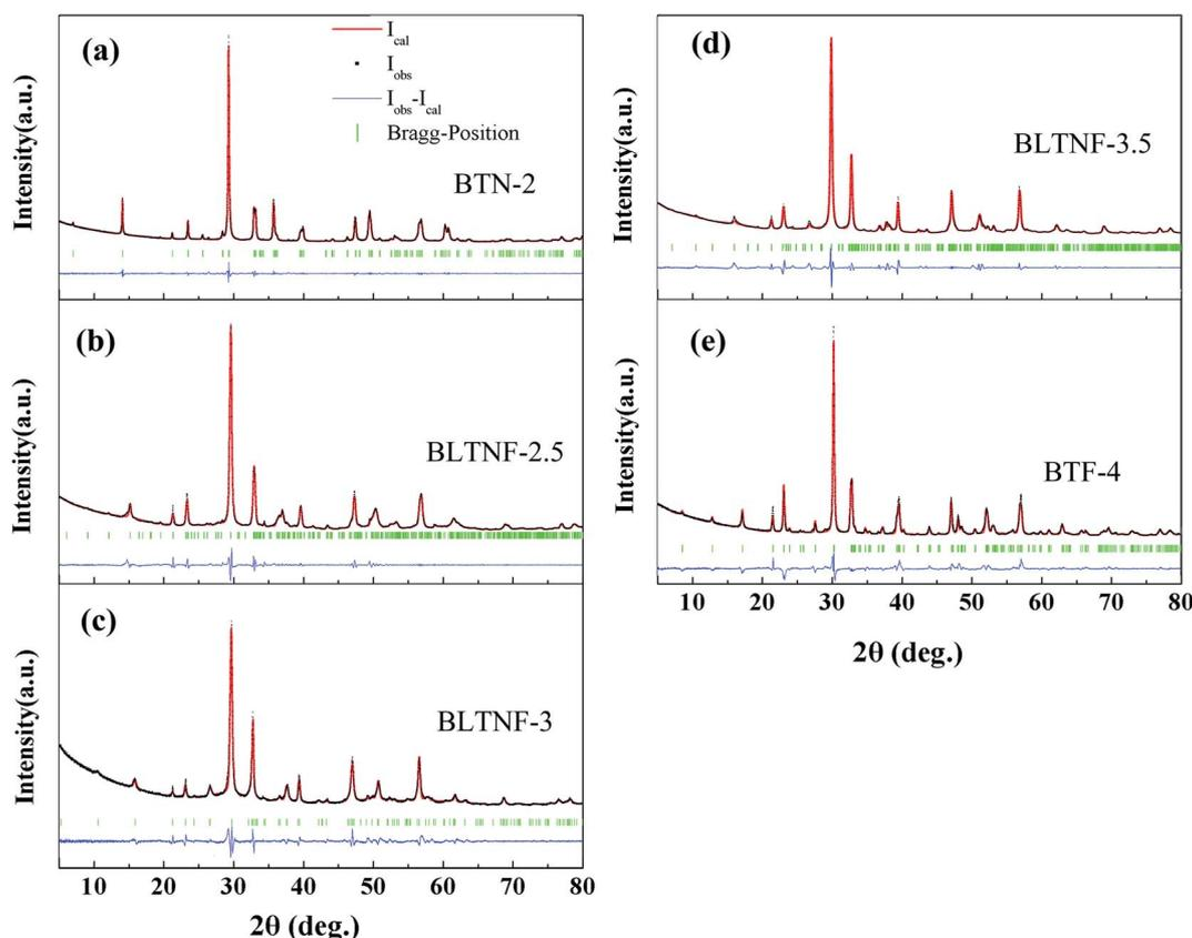
Fig. 2 XRD patterns and refined results of (a)  $\text{Bi}_3\text{TiNbO}_9$  (BTN-2); (b)  $\text{Bi}_3\text{TiNbO}_9\text{-Bi}_3\text{LaTiNbFeO}_{12}$  (BLTNF-2.5); (c)  $\text{Bi}_3\text{LaTiNbFeO}_{12}$  (BLTNF-3); (d)  $\text{Bi}_3\text{LaTiNbFeO}_{12}\text{-Bi}_5\text{Ti}_3\text{FeO}_{15}$  (BLTNF-3.5); and (e)  $\text{Bi}_5\text{Ti}_3\text{FeO}_{15}$  (BTF-4).
