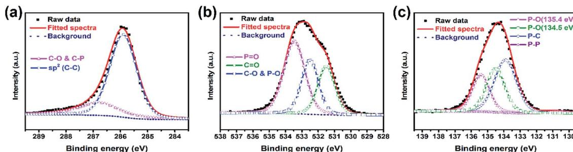
Fig. 4 (a–c) High-resolution C 1s, O 1s and P 2p XPS spectra of P-PBC-70.
