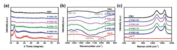
Fig. 2 (a) XRD patterns (b) FT-IR spectra and (c) Raman spectra of red-P, PBC and P-PBC.
