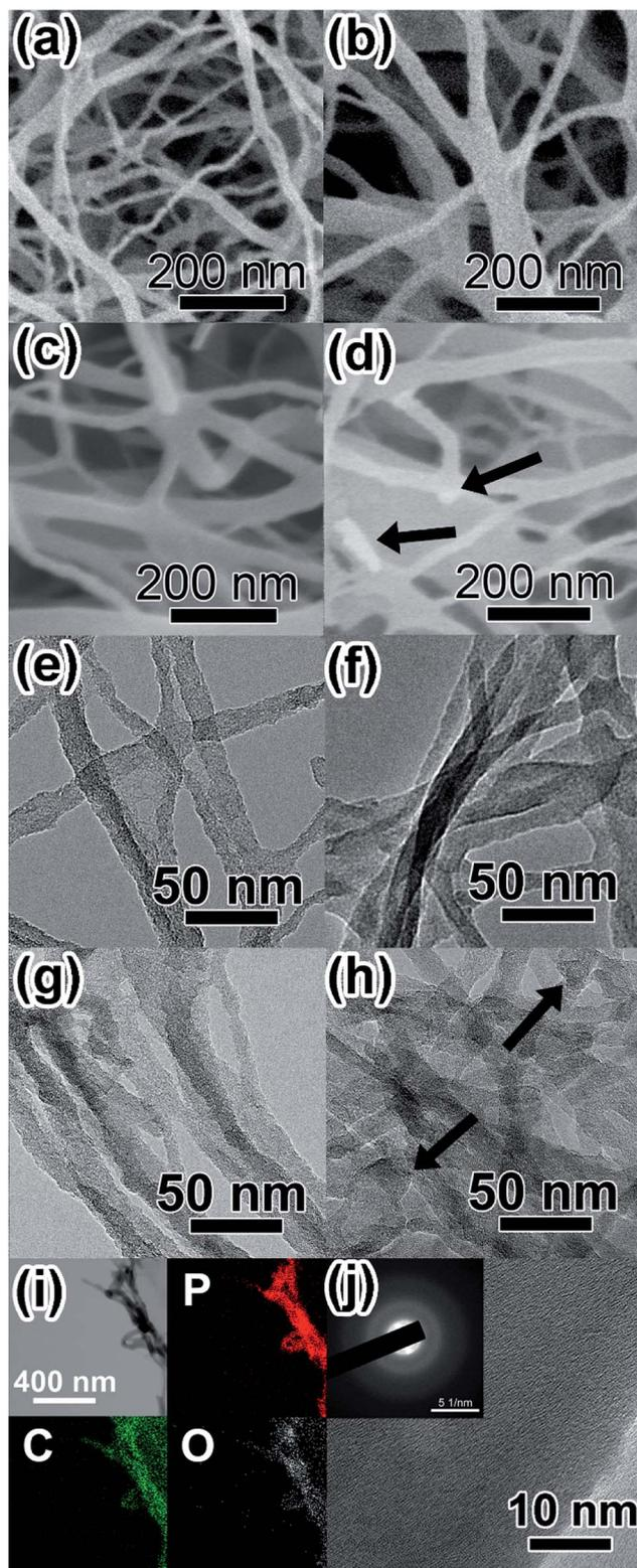
**Fig. 3** (a–d) SEM images and (e–h) TEM images of P-PBC-50, P-PBC-60, P-PBC-70 and P-PBC-80, respectively; (i) elemental mapping images of P, C, and O components; (j) HRTEM image (inset: corresponding SAED pattern with a scale bar of 5 1/nm) of P-PBC-70 composite.
