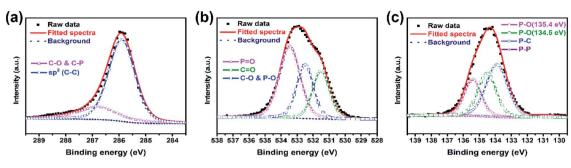
Fig. 4 (a-c) High-resolution C 1s, O 1s and P 2p XPS spectra of P-PBC-70.
