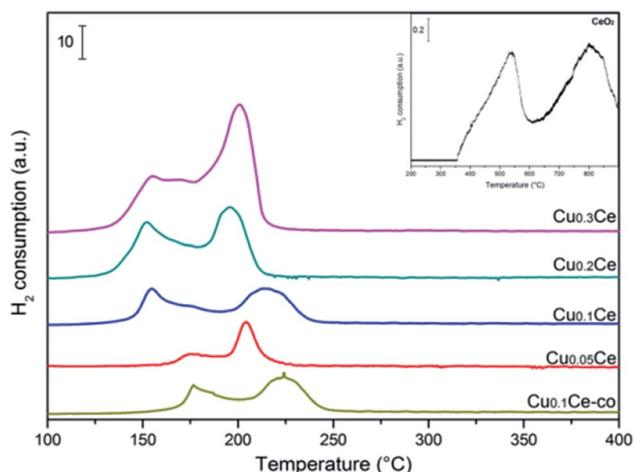
Fig. 6 H<sub>2</sub>-TPR profiles of the various CuCe catalysts.
