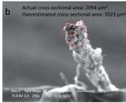
Fig. 3 (a) The paper frames used during the tensile tests; (b) SEM image of GOF@25 $^{\circ}$ -IPA sample after the rupture during the tensile test to calculate their cross-section.
