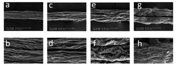
Fig. 5 SEM images of GFs obtained by reducing dried GOF@25 $^{\circ}$ -IPA by different chemical agents:  $500\times$  and  $2000\times$  magnification (a and b) reduced graphene filament by HI/AAc, (c and d) reduced graphene filament by HI, (e and f) reduced graphene filament by AsAc, (g and h) reduced graphene filament by Hdz.
