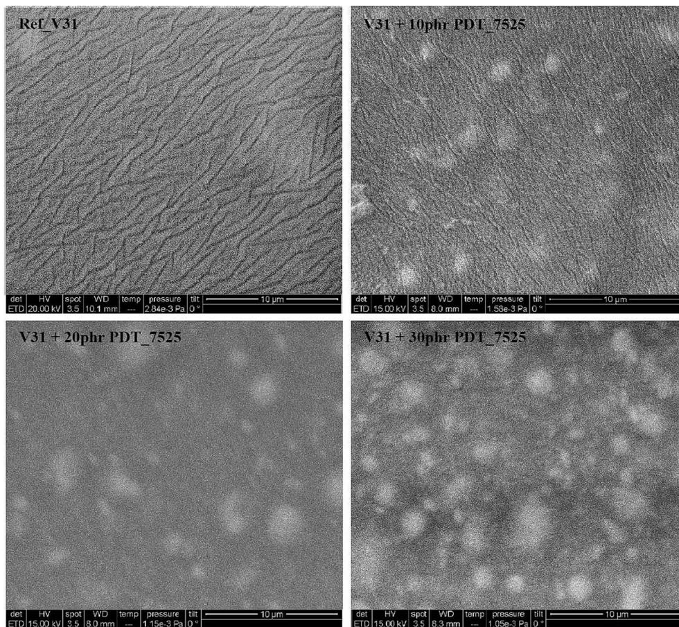
Fig. 2 SEM pictures of elastomers with varying loadings of copolymer PDT\_7525.
