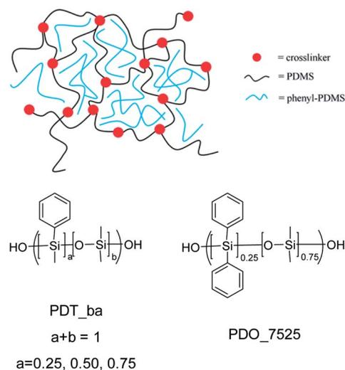
**Scheme 1** Cross-linked elastomer consisting of phenyl-PDMS copolymer in PDMS matrix and structures of the added phenyl-PDMS copolymers.
