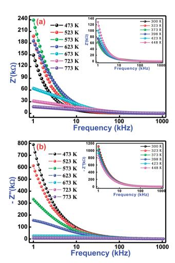
Fig. 5 Variation of (a) real impedance (Z') with frequency and (b) imaginary impedance (Z'') with frequency for Bi(Co<sub>0.40</sub>Ti<sub>0.40</sub>Fe<sub>0.20</sub>)O<sub>3</sub> material at some selected temperatures.
