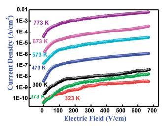
Fig. 9 Variation of current density (J) with electric field (E) relationship at several temperatures of Bi( $Co_{0.40}Ti_{0.40}Fe_{0.20}$ )O<sub>3</sub> material.
