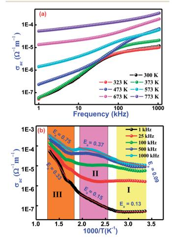
Fig. 8 Variation of (a)  $\sigma_{ac}$  with frequency and (b)  $\sigma_{ac}$  with temperature for Bi(Co<sub>0.40</sub>Ti<sub>0.40</sub>Fe<sub>0.20</sub>)O<sub>3</sub> lead-free material.
