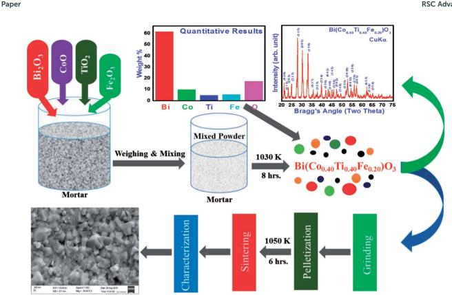
Fig. 1 Schematic syntheses procedure and further characterization of  $Bi(Co_{0.40}Ti_{0.40}Fe_{0.20})O_3$  compound by solid state techniques
