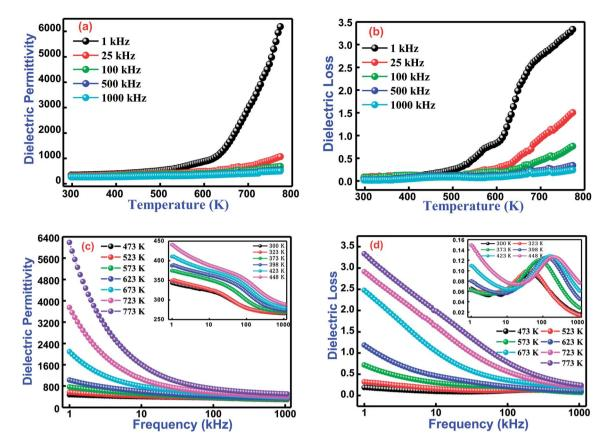
Fig. 4 (a) Temperature dependence dielectric permittivity and (b) dielectric losses at several selected frequencies of  $Bi(Co_{0.40}Ti_{0.44}Fe_{0.20})O_3$  lead free material. (c) Frequencies dependence dielectric permittivity and (d) dielectric loss nature at various selected temperatures (inset shows lower temperature behaviour) for  $Bi(Co_{0.40}Ti_{0.44}Fe_{0.20})O_3$  lead-free material.
