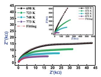
Fig. 6 Nyquist plot of  $Bi(Co_{0.40}Ti_{0.40}Fe_{0.20})O_3$  material at different temperatures. The red solid line denotes fitting with [(CR) (CQR)] equivalent circuit model.
