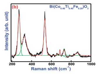
Fig. 2 (a) Room temperature XRD pattern and inset shows Raman spectra and (b) Gaussian fitted Raman spectra of Bi(Co $_{0.40}$ Ti $_{0.40}$ Fe $_{0.20}$ ) O $_3$  lead free material.
