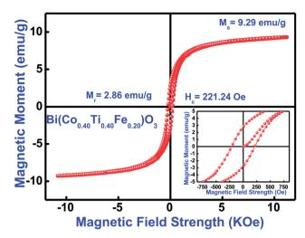
Fig. 10 M-H loops measured at 300 K, (inset) showing enlarged view of Bi(Co<sub>0.40</sub>Ti<sub>0.40</sub>Fe<sub>0.20</sub>)O<sub>3</sub> material.
