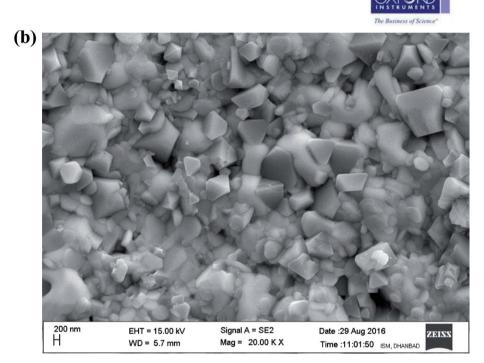
Fig. 3 (a and b) EDXMA analysis and corresponding FE-SEM micrograph of as-sintered Bi( $Co_{0.40}$ Ti<sub>0.44</sub>Fe<sub>0.20</sub>)O<sub>3</sub> compound, respectively, at 300 K.
