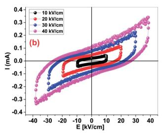
Fig. 11 (a) P-E loops diagram of the Bi(Co<sub>0.40</sub>Ti<sub>0.40</sub>Fe<sub>0.20</sub>)O<sub>3</sub> material. (b) I-E loops diagram of the Bi(Co<sub>0.40</sub>Ti<sub>0.40</sub>Fe<sub>0.20</sub>)O<sub>3</sub> material.
