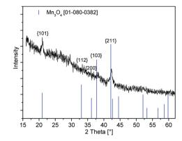
Fig. 4 GIXRD spectra of the as-deposited cobalt oxide (left) and manganese oxide (right) layers by the CCVD process using 4 and 5 as precursors (precursor concentration 0.8 M).
