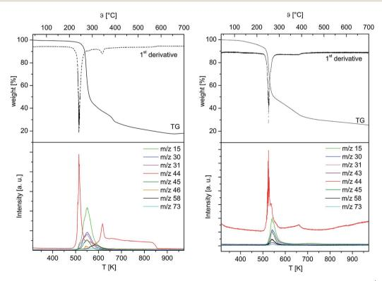
Fig. 3 Thermogravimetry (TG) (top) and selected mass spectrometric scans (bottom) of 4 (left) and 5 (right). m/z = 15 (CH<sub>3</sub><sup>+</sup>), 30 (C<sub>2</sub>H<sub>6</sub><sup>+</sup>), 31 (CH<sub>3</sub>O<sup>+</sup>), 43 (C<sub>2</sub>H<sub>3</sub>O<sup>+</sup>), 44 (CO<sub>2</sub><sup>+</sup>), 45 (C<sub>2</sub>H<sub>6</sub>O<sup>+</sup>), 58 (C<sub>3</sub>H<sub>6</sub>O<sup>+</sup>), 73 (C<sub>4</sub>H<sub>9</sub>O<sup>+</sup>).
