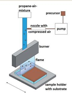
Fig. 1 Schematic CCVD setup.
